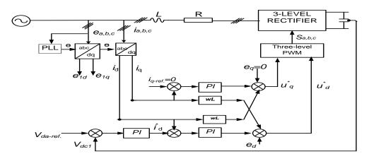
Figure 2. Three-level rectifier controller.
