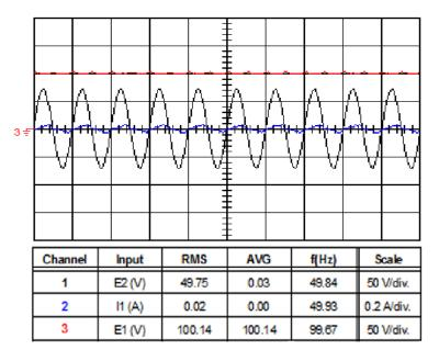
Figure 6. Input voltage input current and output dc voltage
