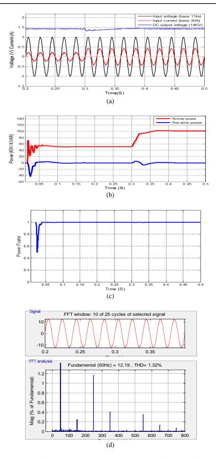
Figure 4. (a) Input voltage, input current and output dc voltage, (b) Active and reactive power, (c) Input power factor and (d) THD on the grid side.
