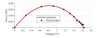
Figure 9: The simulation and experimental characteristic of  $P_{TEG} = f(V_{TEG})$
