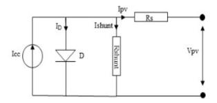
Figure 2. Equivalent diagram of a PV cell under illumination
