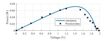
Figure 8. Simulation and experimental characteristic of  $P_{TEG} = f(V_{TEG})$
