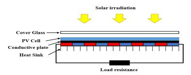
Figure 1. Schematic diagram of a hybrid photovoltaic/thermoelectric system
