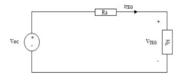
Figure 3. The equivalent diagram of a TEG
