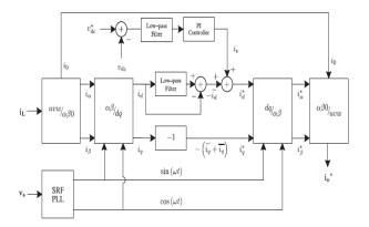
Figure 5. Current reference generator for predictive controller
