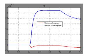
Figure 14. Active and reactive power of STATCOM
