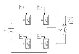
Figure 7. H-bridge with bypass IGBT switch
