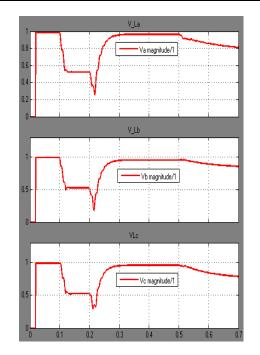
Figure 13.2. Load Voltages of phases during open circuit fault with Controller
