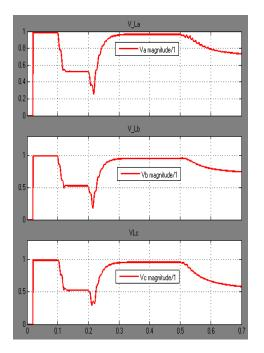
Figure 13.1. Load Voltages of Phases during open circuit fault without Controller
