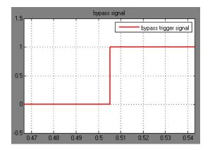
Figure 15. Relay operation signal during open circuit fault at 0.5sec
