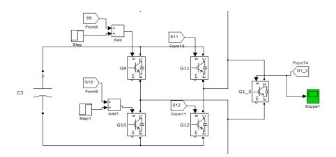
Figure 12. Bypass switch placement with switch fault in S9 and S10 switches
