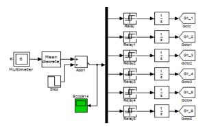
Figure 8. Controller to generate signal for the bypass switches
