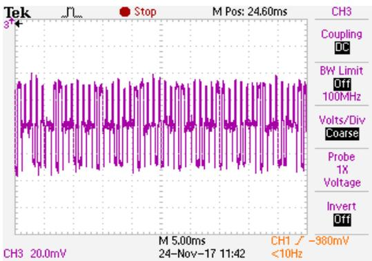
Figure 32. Common Carrier Control Scheme at  $M_i=0.81$ : Common mode voltage :DPWM
