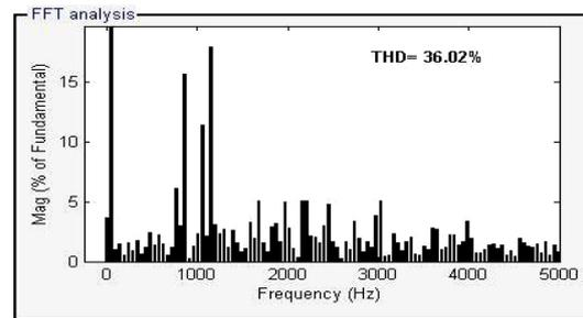
Figure 45. Inverted Phase Shifted Control Scheme at  $M_i=0.81$ : Harmonic distortion of line Voltage along with THD
