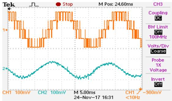
Figure 19. Phase Shifted Control Scheme at  $M_i=0.81$ : Line Voltage and Stator Current :SVPWM
