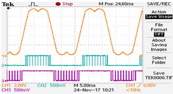
Figure 8. Common Carrier Control Scheme at  $M_i=0.81$ : Modulating Signal, Pulses for Inverter-I & II :SVPWM
