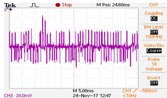
Figure 47. Inverted Phase Shifted Control Scheme at  $M_i=0.81$ : Common mode voltage: DPWM
