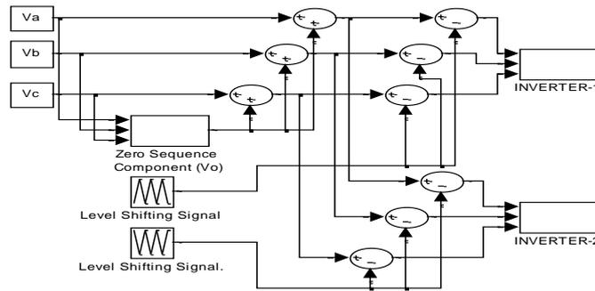
Figure 2. Block diagram illustrating scalar PWM for cascaded three level inverter configuration
