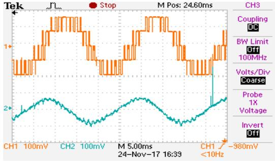
Fig. 39. Phase Shifted Control Scheme at  $M_i=0.81$ : Line Voltage and Stator Current :DPWM
