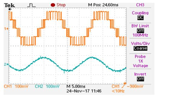
Figure 34. Inverted Carrier Control Scheme at  $M_i=0.81$ : Line Voltage, Stator Current: DPWM
