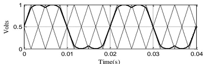
Figure 5. Proposed ICPWM algorithm for cascaded three level inverter
