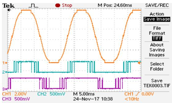
Figure 28. Common Carrier Control Scheme at  $M_i=0.81$ : Modulating Signal, Pulses for Inverter-I & II: DPWM
