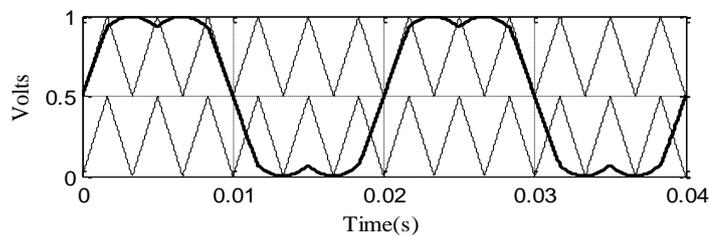
Figure 4. Proposed CCPWM scheme for cascaded three level inverter.
