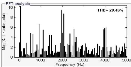
Figure 10. Common Carrier Control Scheme at  $M_i=0.81$ : Harmonic distortion of line Voltage along with THD
