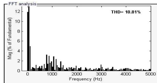
Figure 26. Inverted Phase Shifted Control Scheme at  $M_i=0.81$ : Harmonic distortion of stator current along with THD
