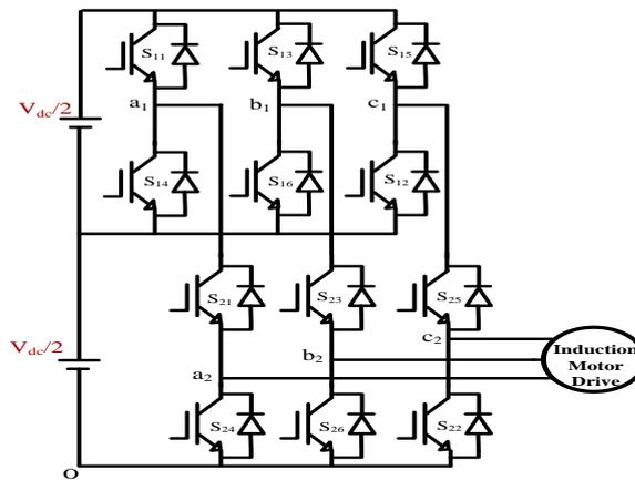
Figure 1. Proposed three-level cascaded inverter configuration
