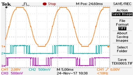
Figure 38. Phase Shifted Control Scheme at  $M_i=0.81$ : Modulating Signal, Pulses for Inverter-I & II :DPWM
