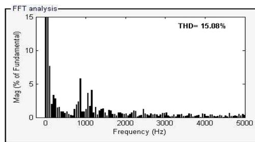
Figure 46. Inverted Phase Shifted Control Scheme at  $M_i=0.81$ : Harmonic distortion of stator current along with THD
