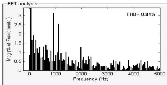
Figure 31. Common Carrier Control Scheme at  $M_i=0.81$ : Harmonic distortion of stator current along with THD
