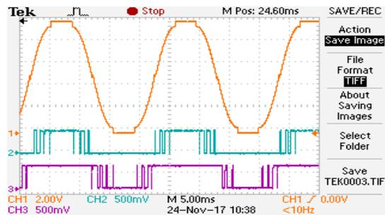
Figure 43. Inverted Phase Shifted Control Scheme at  $M_i=0.81$ : Modulating Signal, Pulses for Inverter-I & II: DPWM
