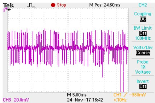
Figure 42. Phase Shifted Control Scheme at  $M_i=0.81$ : Common mode voltage :DPWM
