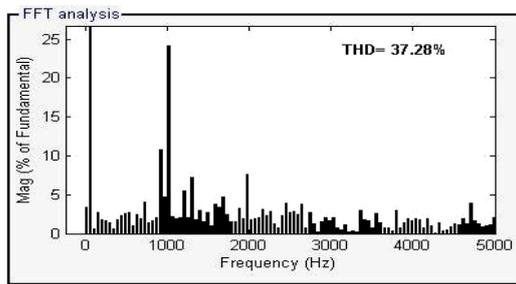
Figure 40. Phase Shifted Control Scheme at  $M_i=0.81$ : Harmonic distortion of line Voltage along with THD
