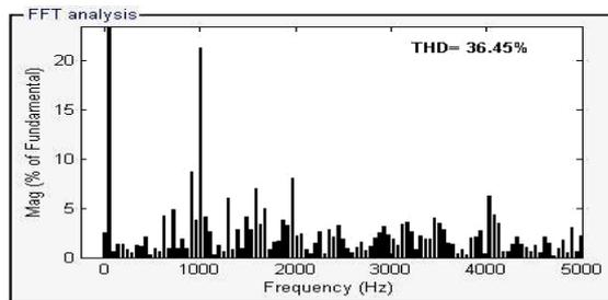
Figure 20. Phase Shifted Control Scheme at  $M_i=0.81$ : Harmonic distortion of line Voltage along with THD
