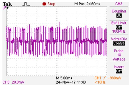
Figure 37. Inverted Carrier Control Scheme at  $M_i=0.81$ : Common mode voltage :DPWM
