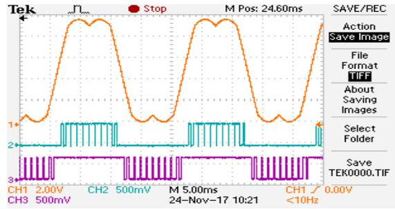
Figure 13. Inverted Carrier Control Scheme at  $M_i=0.81$ : Modulating Signal, Pulses for Inverter-I & II :SVPWM
