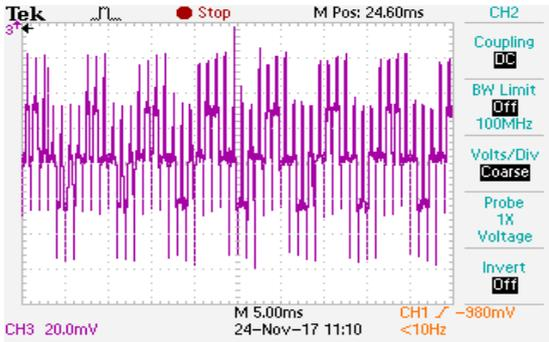
Figure 12. Common Carrier Control Scheme at  $M_i=0.81$ : Common mode voltage :SVPWM
