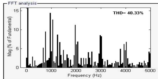
Figure 15. Inverted Carrier Control Scheme at  $M_i=0.81$ : Harmonic distortion of line Voltage along with THD
