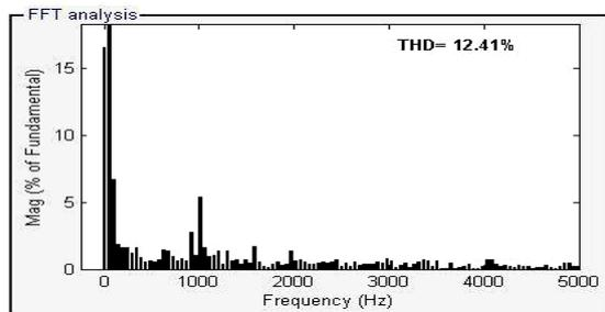
Figure 21. Phase Shifted Control Scheme at  $M_i=0.81$ : Harmonic distortion of stator current along with THD
