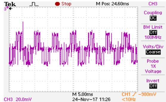
Figure 17. Inverted Carrier Control Scheme at  $M_i=0.81$ : Common mode voltage :SVPWM
