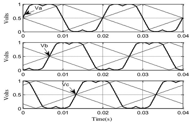
Figure 7. Proposed IPSPWM algorithm for cascaded three level inverter as shown below and cited in the manuscript
