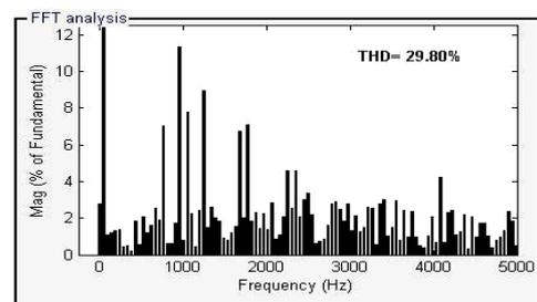
Figure 30. Common Carrier Control Scheme at  $M_i=0.81$ : Harmonic distortion of line Voltage along with THD
