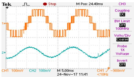
Figure 29. Common Carrier Control Scheme at  $M_i=0.81$ : Line Voltage, Stator Current: DPWM
