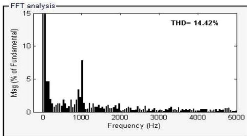
Figure 41. Phase Shifted Control Scheme at  $M_i=0.81$ : Harmonic distortion of stator current along with THD
