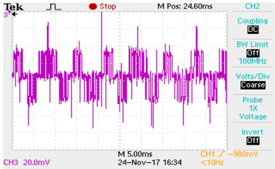
Figure 22. Phase Shifted Control Scheme at  $M_i=0.81$ : Common mode voltage :SVPWM
