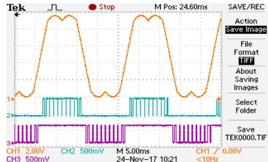
Figure 23. Inverted Phase Shifted Control Scheme at  $M_i=0.81$ : Modulating Signal, Pulses for Inverter-I & II :SVPWM
