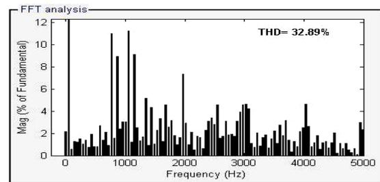
Figure 25. Inverted Phase Shifted Control Scheme at  $M_i=0.81$ : Harmonic distortion of line Voltage along with THD
