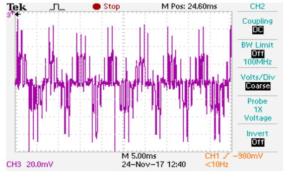
Figure 27. Inverted Phase Shifted Control Scheme at  $M_i=0.81$ : Common mode voltage: SVPWM
