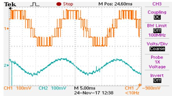
Figure 24. Inverted Phase Shifted Control Scheme at  $M_i=0.81$ : Line Voltage and Stator Current :SVPWM
