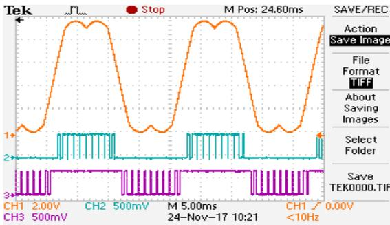
Figure 18. Phase Shifted Control Scheme at  $M_i=0.81$ : Modulating Signal, Pulses for Inverter-I & II :SVPWM
