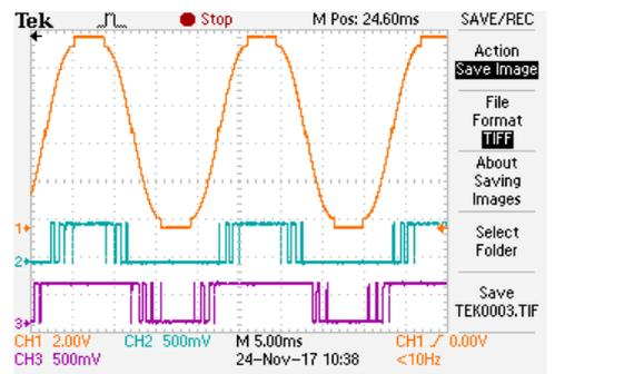
Figure 33. Inverted Carrier Control Scheme at  $M_i=0.81$ : Modulating Signal, Pulses for Inverter-I & II :DPWM
