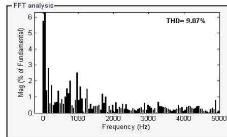
Figure 36. Inverted Carrier Control Scheme at  $M_i=0.81$ : Harmonic distortion of stator current along with THD
