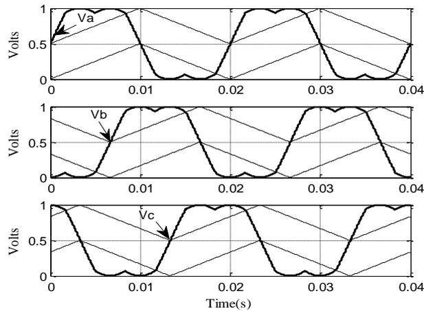
Figure 6. Proposed PSPWM algorithm for cascaded three level inverter.
