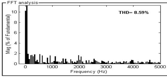
Figure 11. Common Carrier Control Scheme at  $M_i=0.81$ : Harmonic distortion of stator current along with THD
