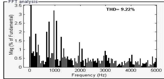
Figure 16. Inverted Carrier Control Scheme at  $M_i=0.81$ : Harmonic distortion of stator current along with THD
