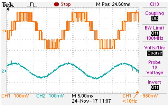
Figure 9. Common Carrier Control Scheme at  $M_i=0.81$ : Line Voltage, Stator Current :SVPWM
