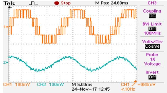
Figure 44. Inverted Phase Shifted Control Scheme at  $M_i=0.81$ : Line Voltage and Stator Current: DPWM
