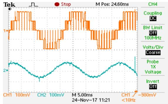
Figure 14. Inverted Carrier Control Scheme at  $M_i=0.81$ : Line Voltage, Stator Current :SVPWM
