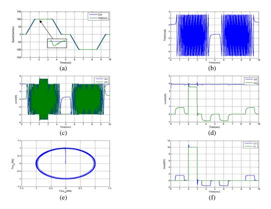
Figure 6. simulation results of sensorless performance of induction motor drive with PMRAS observer (a) rotor speed, (b) rotor position, (c) phase current, (d) d & q axis stator currents, (e) alpha & beta axis rotor fluxes, (f) torque
