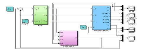
Figure 5. Block diagram of sensorless induction motor drive with CMRAS/ PMRAS speed observers
