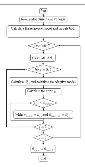
Figure 4. The rotor position search algorithm
