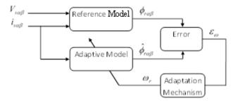
Figure 1. The classical rotor flux MRAS observer
