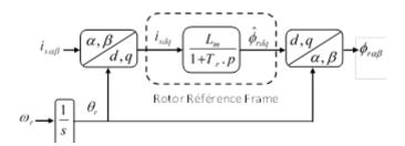
Figure 2. The Adaptaive model in the rotor reference frame
