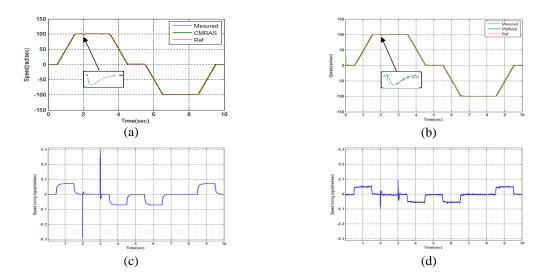
Figure 7. Simulation results of comparative sensorless performance of induction motor drive between CMRAS and PMRAS observers (a) rotor speed CMRAS, (b) rotor speed PMRAS, (c) speed error CMRAS, (d) speed error PMRAS
