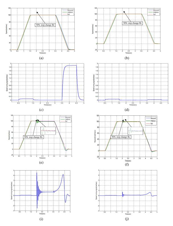
Figure 8. Simulation results of sensorless performance of induction motor drive with impact of rotor and stator resistances change. (a,e) rotor speed CMRAS, (b,f) rotor speed PMRAS, (c,i) speed error CMRAS, (d,j) speed error PMRAS
