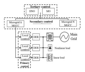
Figure 2. Hierarchical structure of microgrid control system
