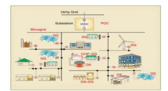
Figure 1. Microgrid structure layout with loads and distributed energy resources (DER) units
