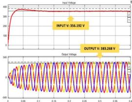
Figure 4. Input and output voltage with 10kW load
