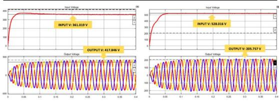
Figure 8. Input and output voltage with 1 p.u reference voltage value
