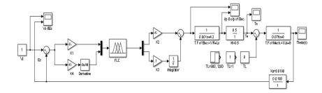
Figure 11. Simulink model of I.M with (fuzzy-PI) Controller
