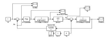
Figure 10. Simulink model of I.M with PI- Controller
