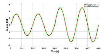
Figure 9. The step response signal with Iref = 3.2A at 0.04s and Iref = 5A at 0.08s
