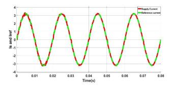
Figure 7. Input current keep track the reference signal by applying APF with HCC
