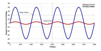
Figure 6. Sinusoidal input current in phase with the voltage waveforms
