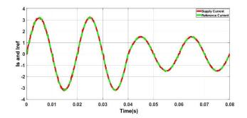
Figure 8. The step response signal with Iref = 3.2A at 0.04s and Iref = 1.5A at 0.08s
