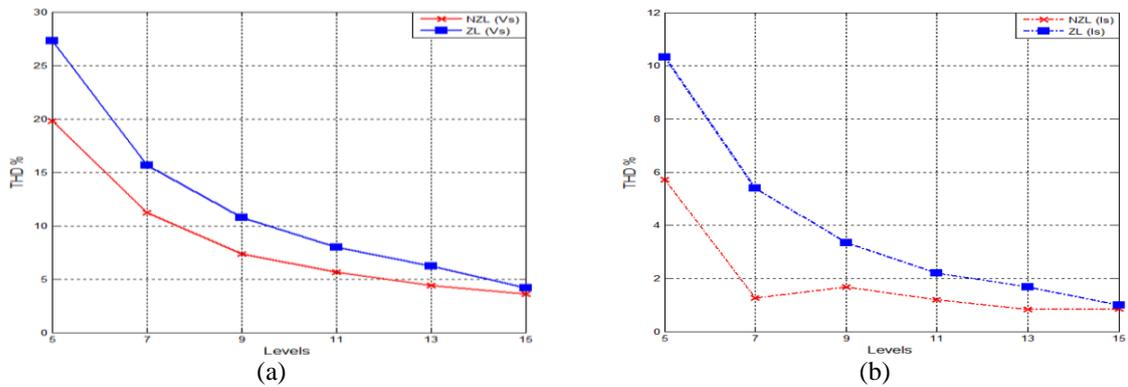
Figure 6. THD of the, (a) MI voltage, (b) current of the proposed MI with NZL and ZL states
