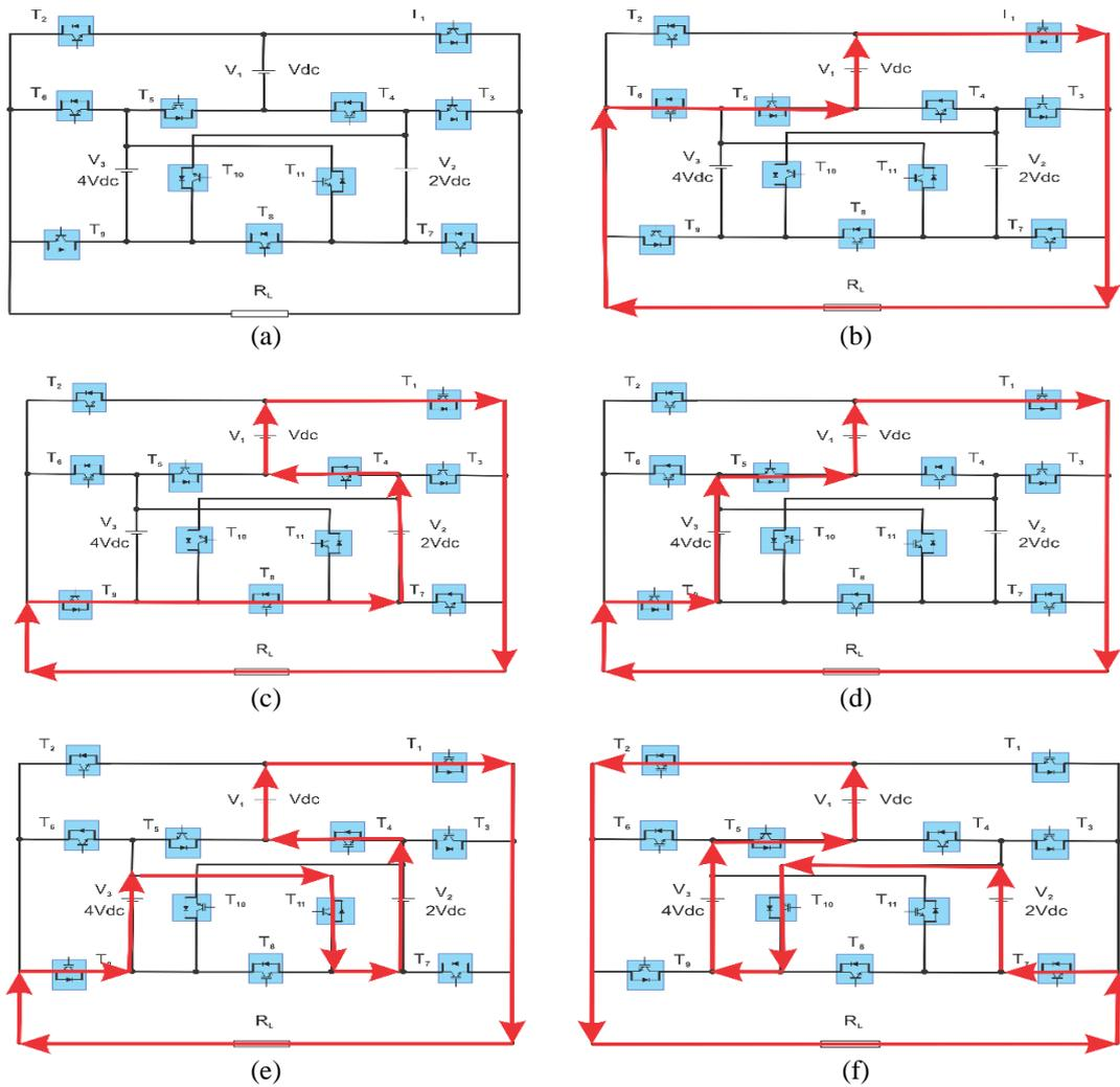
Figure 2. These figures are, (a) modeling of new proposed 15-level inverter topology, (b) selected path configuration with load voltage of  $V_{dc}$ , (c)  $3 V_{dc}$ , (d)  $5 V_{dc}$ , (e)  $7 V_{dc}$ , (f)  $-7 V_{dc}$
