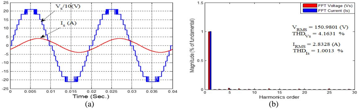
Figure 4. (a) Output MI voltage and current, and (b) spectrum analyzer of the 15-level inverter with ZL state
