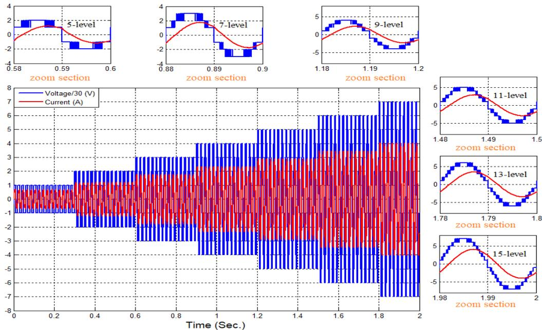
Figure 7. Different output voltage and current of the proposed MI with NZL
