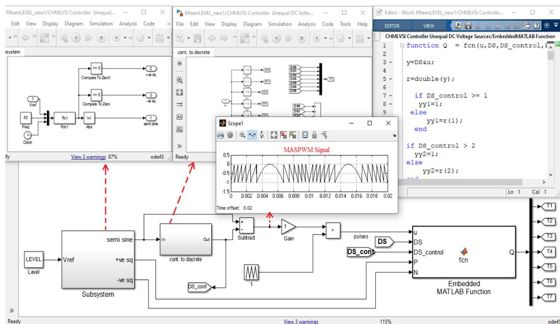
Figure 3. Control circuit of the proposed MI
