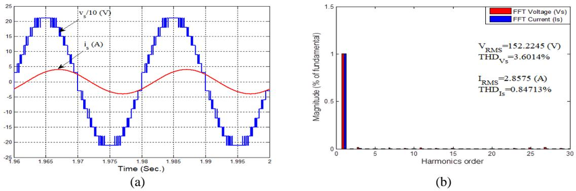
Figure 5. (a) Output MI voltage and current, and (b) spectrum analyzer of the 15-level inverter with NZL state
