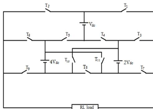
Figure 1. Proposed 15-level inverter topology
