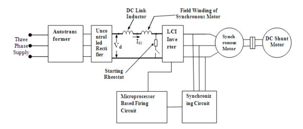
Figure 1. Block diagram of the SCR inverter fed three-phase synchronous motor
