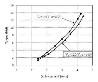
Figure 2. Variation of torque with dc link current for different values of dc link voltage and firing angle
