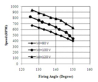
Figure 4. Variation of machine speed with firing angle for different values of dc link voltage
