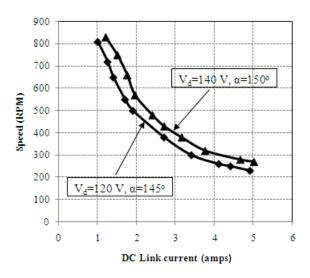
Figure 3. Variation of machine speed with input dc current to the inverter
