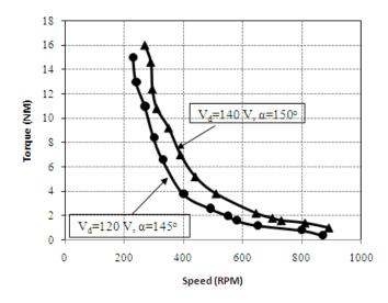
Figure 1. Variation of torque with machine speed for different values of dc link voltage and firing angle
