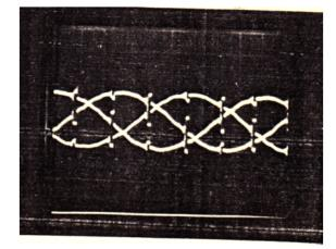
Figure 5. Waveforms of machine Terminal voltages  $V_{ab}$ ,  $V_{bc}$  and  $V_{ca}$
