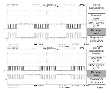
Fig.17. Phase R pulses from DSP Controller.
