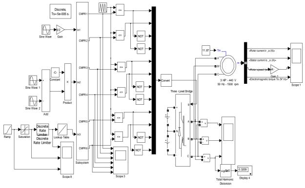
Fig.9. Simulink block of Scalar Control
