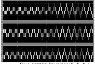
Fig 14. output line-line voltages (V<sub>ab</sub>.V<sub>bc</sub>,V<sub>ca</sub>)
