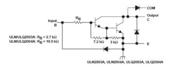
Fig.18. Circuit diagram of Level shifter
