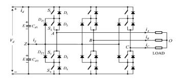
Fig 1. Three-level NPC inverter
