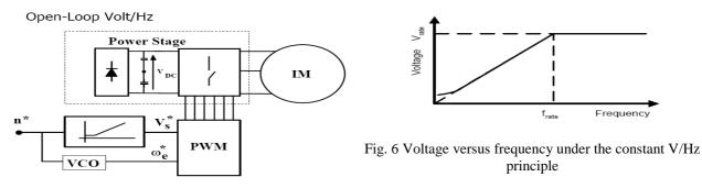
Fig 5 Open -Loop Volt/Hz
