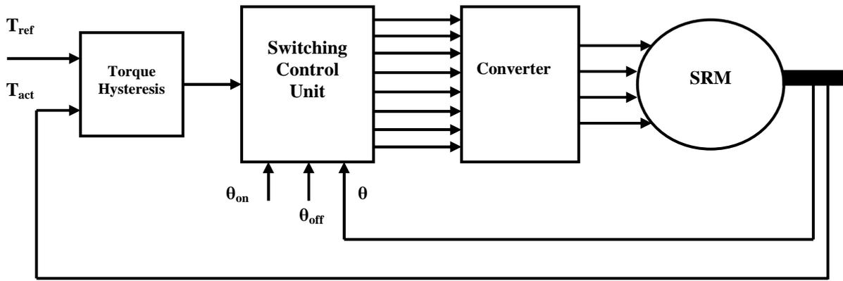
Figure 2. Block diagram of DITC
