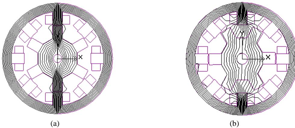
Figure 3. Flux plots of FEA (a) Aligned position (b) Unaligned position
