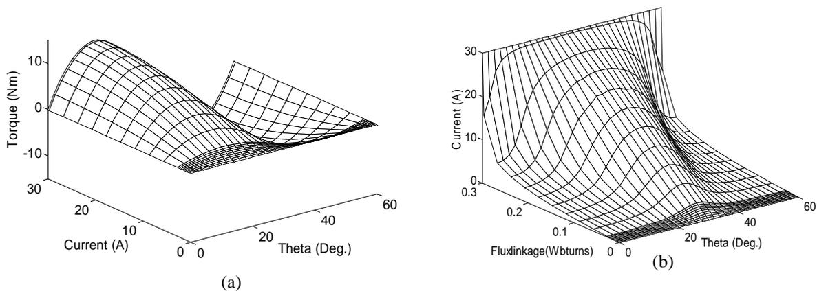
Figure 4. Mesh plots (a) position-current-torque (b) position-flux linkage-current
