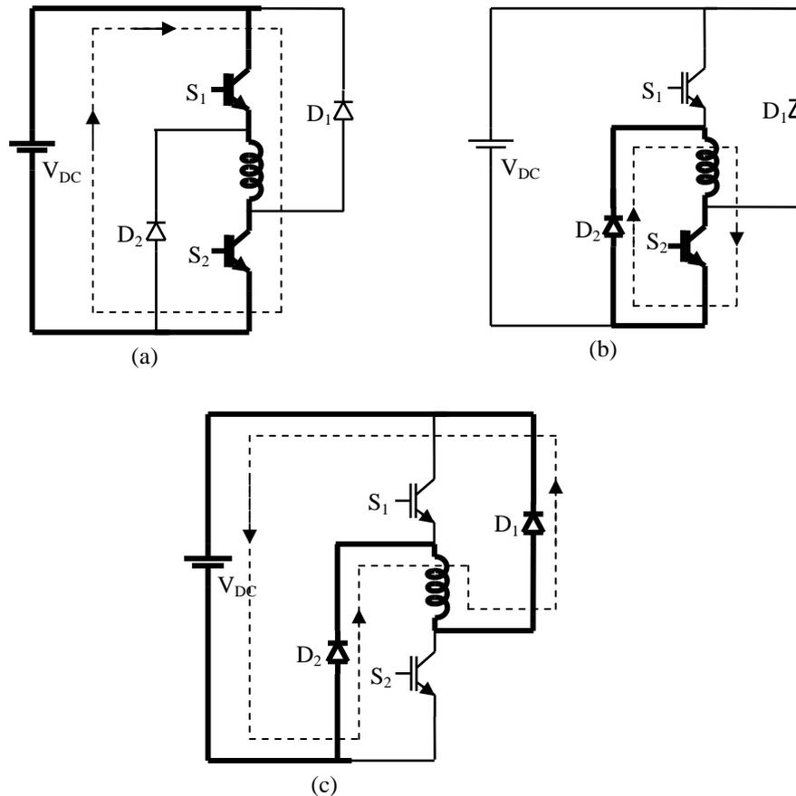
Figure 1. SRM voltage states (a) state 1 (b) state 0 (c) state -1
