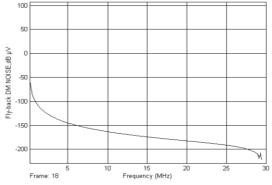
Figure 7 DM noise generated by a simulated Flyback Converter with 47  $\mu$ F bulk filter capacitor
