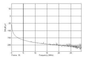
Figure 13 DM noise generated by a simulated Soft Switching Fly-back Converter having 47  $\mu$ F bulk filter capacitor with 0.287 ESR and 22nH ESL
