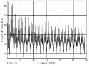
Figure 5 DM noise generated by a simulated Forward Converter with 47 μF bulk filter capacitor with
