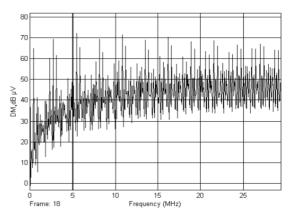
Figure 15 DM noise generated by a simulated Soft Switching Fly-back Converter having 47 μF bulk filter capacitor with 0.287 ESR, 22nH ESL, 12nH path inductance and 150pF MOSFET drain to earth capacitance
