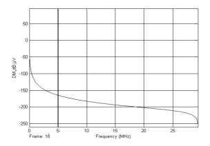
Figure 12 DM noise generated by a simulated Soft Switching Fly-back converter with a 47µF Bulk Filter Capacitor
