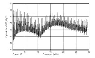
Figure 10 DM noise generated by a simulated Flyback converter having a Bulk Filter capacitor of 47  $\mu$ F with 22 nH ESL, 0.287  $\Omega$  ESR, a 12nH path inductance and a 150pF capacitor added representing the stray capacitor between MOSFET switch drain and earth terminal
