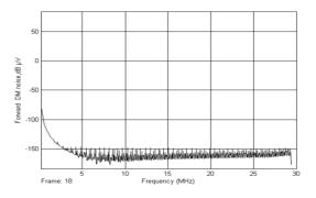
Figure 3 DM noise generated by a simulated Forward Converter with 47 μF bulk filter capacitor with 0.287 Ω ESR and 22nH ESL
