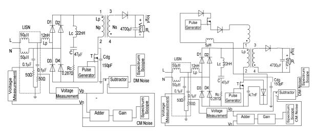
Figure 1(b) Block diagram of a Fly-back converter and noise measurement set-up including LISN
