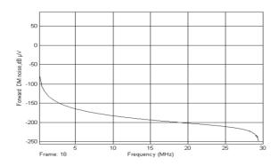
Figure 2 DM noise generated by a simulated Forward Converter with 47  $\mu F$  bulk filter capacitor
