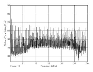
Figure 17 Total Noise generated by a simulated Flyback converter with a 150pF capacitor added between MOSFET switch drain and earth terminal
