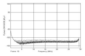
Figure 9 DM noise generated by a simulated Flyback converter having a Bulk Filter capacitor of 47  $\mu$ F with 22 nH ESL and 0.287  $\Omega$  ESR and a 12nH path inductance
