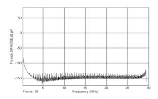
Figure 8 DM noise generated by a simulated Fly-back Converter having 47  $\mu$ F bulk filter capacitor with 0.287  $\Omega$  ESR and 22nH ESL
