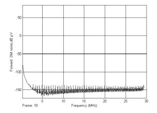
Figure 4 DM noise generated by a simulated Forward Converter with 47  $\mu$ F bulk filter capacitor with 0.287  $\Omega$  ESR and 22nH ESL and 12 nH path inductance
