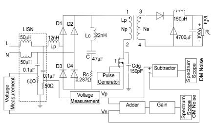
Figure 1(a) Block diagram of a Forward converter and noise measurement set-up including LISN
