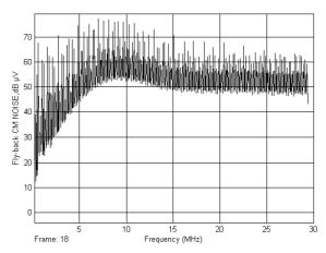
Figure 11 CM noise generated by a simulated Flyback converter with a 150pF capacitor added between MOSFET switch drain and earth terminal
