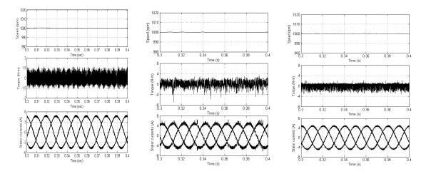
Figure 5. Steady state plots of CSVPWM, AZSPWM1 and AZSPWM2 algorithms based vector controlled induction motor drive respectively
