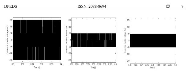
Figure 7. Common mode voltage variations in CSVPWM, AZSPWM1 and AZSPWM2 algorithms based vector controlled induction motor drive respectively
