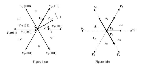
Figure 1 (a) Possible voltage space vectors and sector definition in CSVPWM algorithm (b) Voltage space vectors and formation of AZSPWM algorithms
