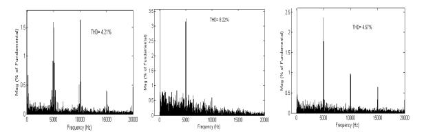
Figure 6. Harmonic spectra of line current in CSVPWM, AZSPWM1 and AZSPWM2 algorithms based vector controlled induction motor drive respectively
