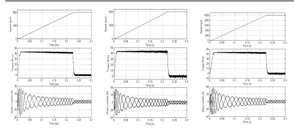
Figure 4. Starting transients of CSVPWM, AZSPWM1 and AZSPWM2 algorithms based vector controlled induction motor drive respectively
