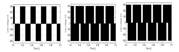
Figure 3. Line voltages of CSVPWM, AZSPWM1 and AZSPWM2 algorithms based vector controlled induction motor drive respectively
