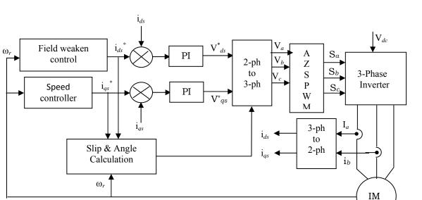
Figure 2. Block diagram of proposed AZSPWM algorithms based vector controlled induction motor
