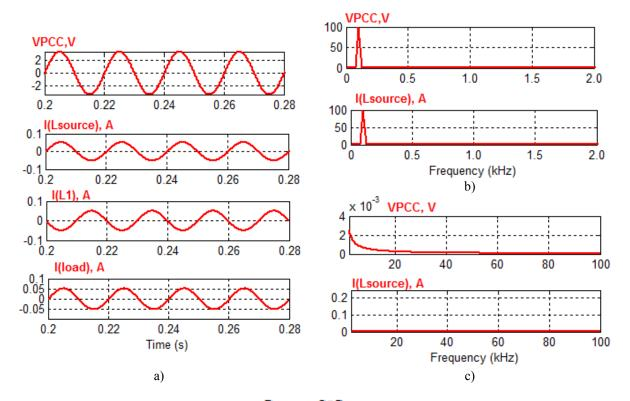
Figure 5. Simulation results when the load is  $R_{load} = 33\Omega$ . a) time domain from top to bottom: voltage of the PCC, grid current, inverter current, and load current; b) harmonic spectrum analysis of the voltage of the PCC and source current from 0 to 2kHz; c) harmonic spectrum analysis voltage of the PCC and source current from 2 to 100kHz
