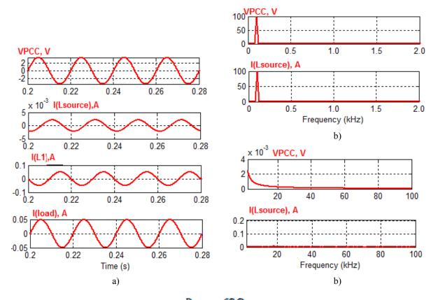
Figure 4. Simulation results when the load is  $R_{load} = 68 \Omega$ . a) time domain from top to bottom: voltage of the PCC, grid current, inverter current, and load current; b) harmonic spectrum analysis of the voltage of the PCC and source current from 0 to 2 kHz; c) harmonic spectrum analysis voltage of the PCC and source current from 2 to 100kHz
