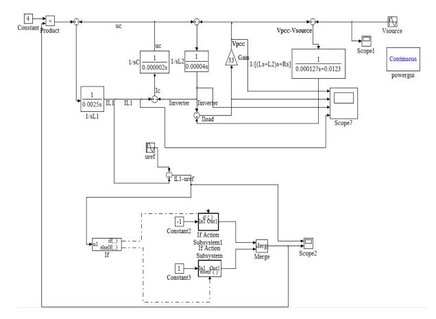
Figure 3. Simulation model of fuzzy-logic hysteresis control of single-phase grid inverter
