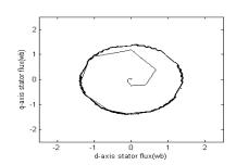
Figure 9. Conventional DTC: Locus of Stator Flux
