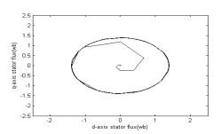
Figure 10. Proposed DTC: Locus of Stator Flux
