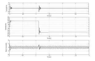
Figure 15. Conventional DTC: Transients during Speed Reversal
