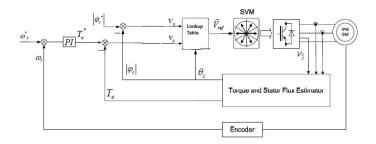
Figure 3. Conventional DTC Applied to PMSM
