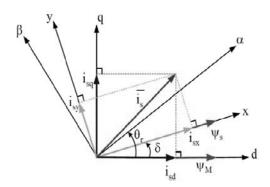
Figure 1. Stator and Rotor Magnetic Fluxes in Various Reference Frames
