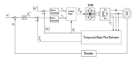
Figure 4. Implementation of Neuro Controllers in DTC of PMSM
