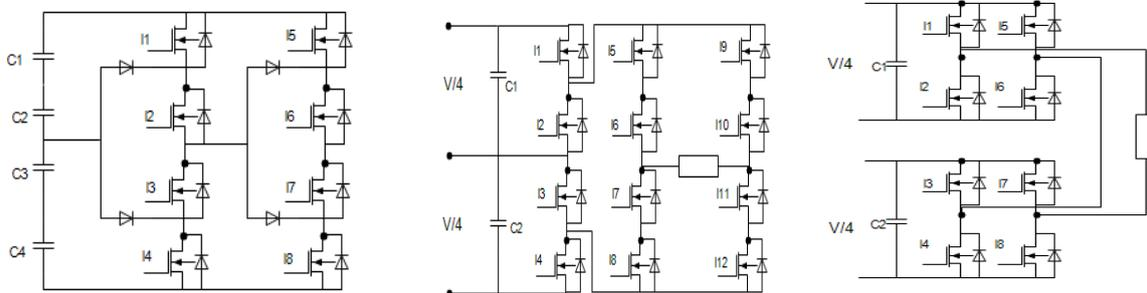
Figure 3(a), (b),(c). Five level Multi level clamped MLI, Reverse voltage MLI, cascaded MLI
