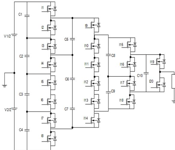
Figure 2. Five Levels generalized multi-level inverter
