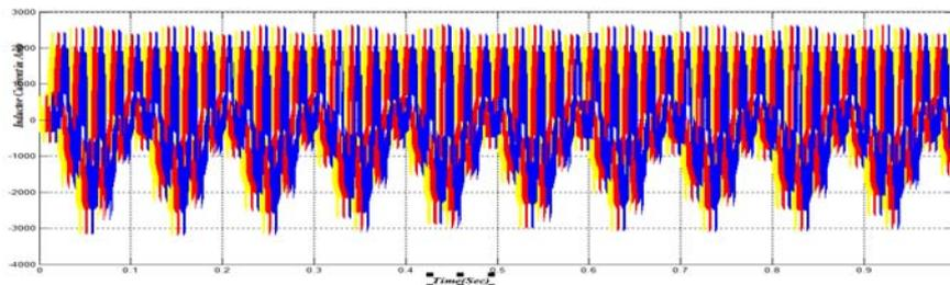
Figure 7. Inductor currents is a five level MMI by using Sinusoidal Pulse width modulation technique
