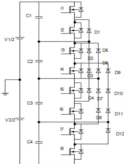
Figure 1. Five Level diode clamped multi-level inverter
