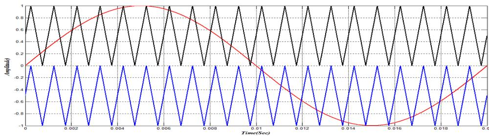
Figure 5. Sinusoidal Pulse width modulation technique.
