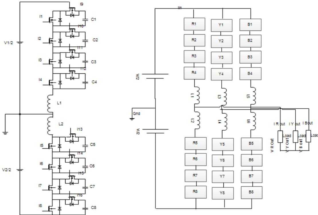
Figure 4. Five Level Modular MLI with chopper cells and details of its three phase system
