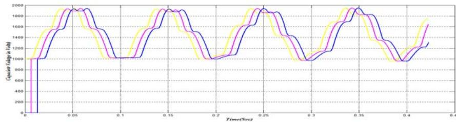
Figure 6. Capacitor currents is a five level MMI by using Sinusoidal Pulse width modulation technique
