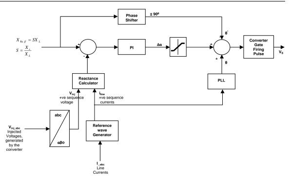
Figure 9. Basic Control Block for SSSC
