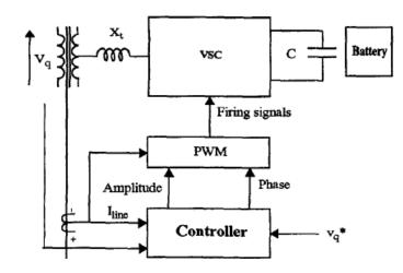
Figure 8. Basic Control block of SSSC
