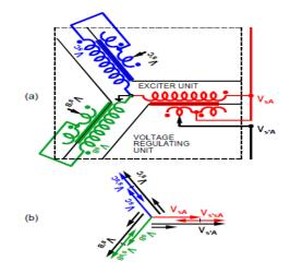
Figure 2. (a) Voltage regulator circuit (b) phasor diagram
