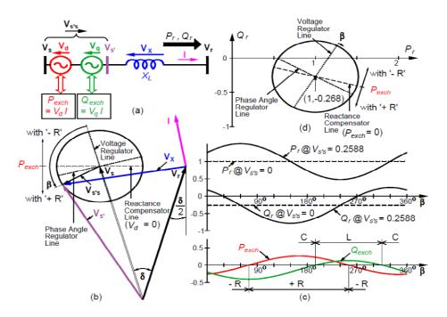
Figure 4. Effect of a series-connected voltage source on power flow in a transmission Line. (a) Power transmission system with a series-connected compensating voltage, Vs's, (b) phasor diagram,
