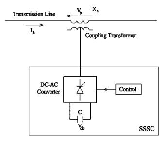
Figure 1. Basic Building block of SSSC
