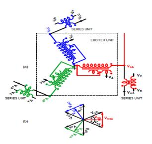
Figure 3. (a) Phase angle regulator circuit (b) phasor diagram
