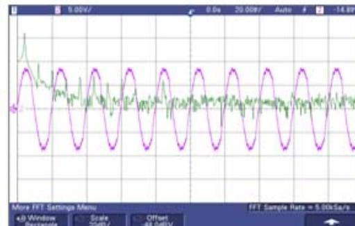
Figure 6. Voltage waveform and its FFT analysis
