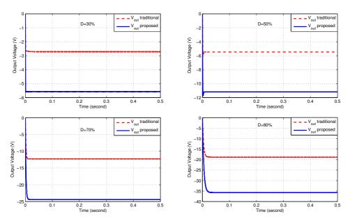
Figure 12. Output voltage of simulink model compared with traditional buck boost circuit with D=30%, 50%, 70%, and 80%
