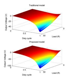
Figure 11. System's output with different load and duty cycle
