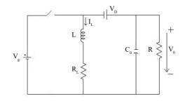
Figure 7. Traditional buck boost converter's equivalent circuit in OFF state
