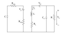
Figure 9. Switched capacitor buck boost converter's equivalent circuit in OFF state
