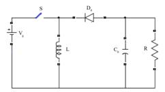
Figure 1. Traditional buck boost converter
