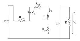
Figure 8. Switched capacitor buck boost converter's equivalent circuit in ON state
