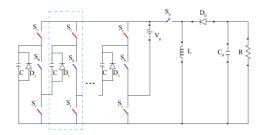
Figure 2. Switched-capacitor buck-boost converter with high voltage gain
