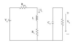
Figure 6. Traditional buck boost converter's equivalent circuit in ON state
