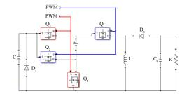
Figure 3. One stage switched-capacitor buck-boost converter
