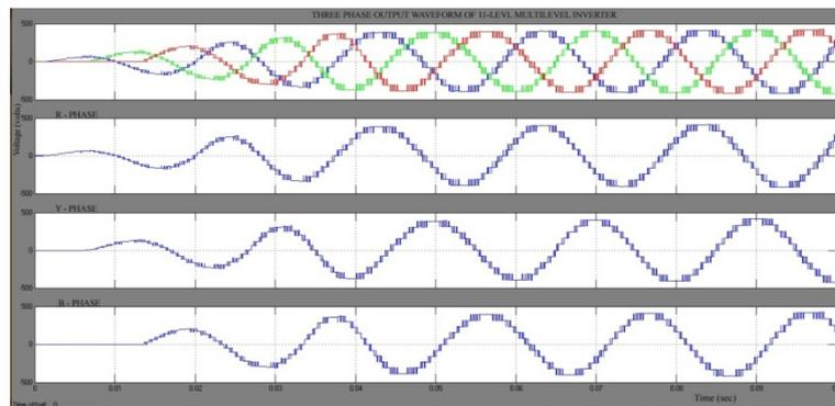
Figure 4(a). Output voltage of three phase Cascaded 11 level inverter with PV cells
