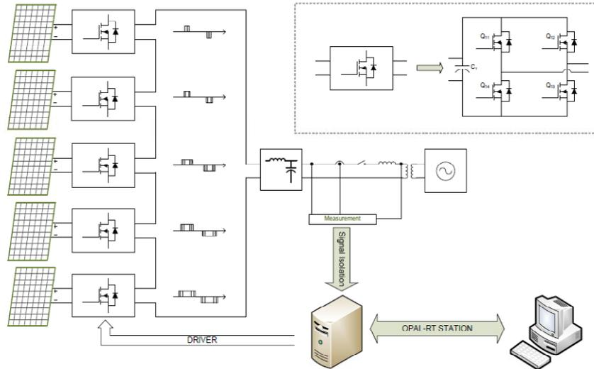
Figure 2. Multilevel inverter system overview
