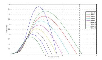
Figure 2. The typical curves of Cp versus  $\lambda$  for various values of the pitch angle  $\beta$
