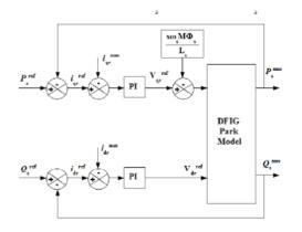
Figure 3. Power control of the DFIG
