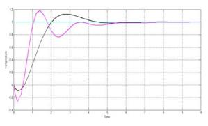
Figure 8. Comparison of ZN and MZN tuned PI controller
