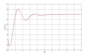
Figure 3. Set point tracking of CSTR process with ZN PI controller
