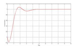
Figure 6. Set point tracking of CSTR process with Tyreus-Luyben tuning PI controller
