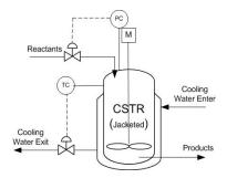
Figure 1. The Schematic of a CSTR
