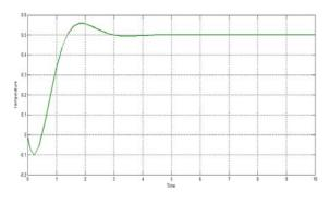
Figure 7. Set point tracking of CSTR process with IMC Based tuned PI controller
