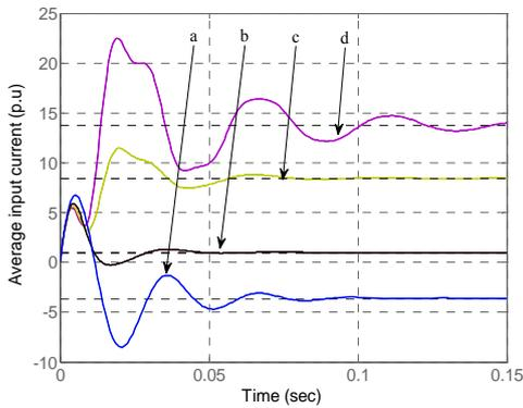
Figure 4. Step response of the average input current (p.u.) for two parallel-connected inverters with null grid resistance and different values of line resistance: a-  $0.5\Omega$ , b-  $0.2\Omega$ , c-  $0.1\Omega$ , d-  $0.05\Omega$
