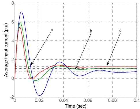
Figure 5. Step response of the input current (p.u.) for a given number of parallel-connected inverters: a-  $n=1$ ; b-  $n=2$  and c-  $n=3$
