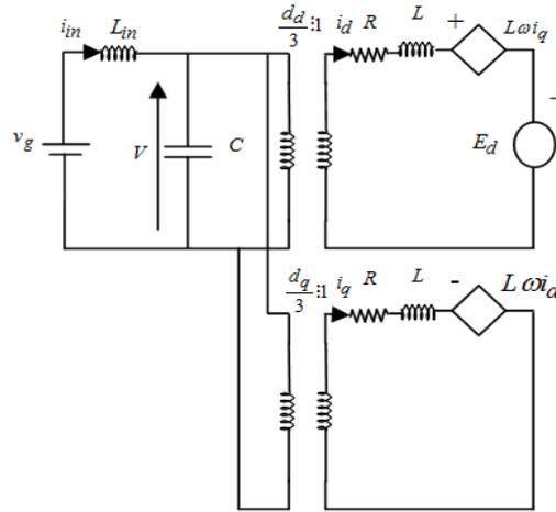
Figure 3. A simplified average equivalent circuit model
