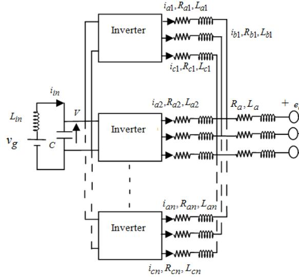
Figure 1. Circuit structure for the  $n$ -parallel connected inverters
