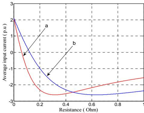
Figure 6. Line and grid resistance effects on the steady state input current (p.u): a) variation of  $R_g$ , b) variation of  $R_l$
