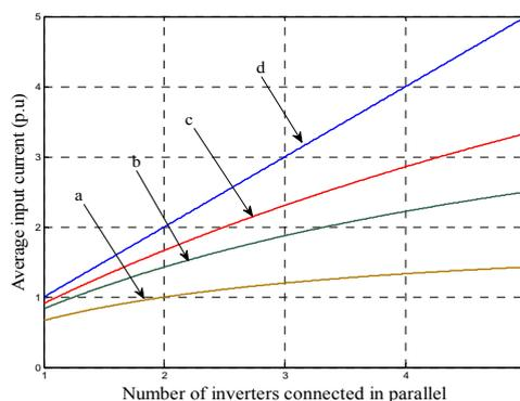
Figure 8. Average input current(p.u) with respect to the number  $n$  of parallel connected inverters with different grid impedance ( $R_g, L_g$ ): a-  $0.05 \Omega$ ,  $0.17 \text{ mH}$ ; b-  $0.02 \Omega$ ,  $0.068 \text{ mH}$ ; c-  $0.01 \Omega$ ,  $0.034 \text{ mH}$ ; d-  $0 \Omega$ ,  $0 \text{ mH}$
