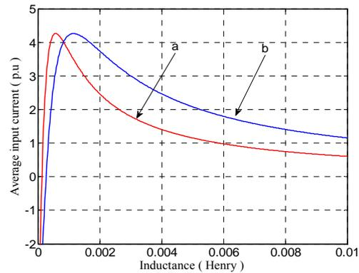
Figure 7. Line and grid inductance effects on the  $R_g$  steady state input current (p.u): a) variation of  $L_g$ , b) variation of  $L_l$
