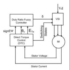
Figure 9. Block diagram of fuzzy duty ratio control
