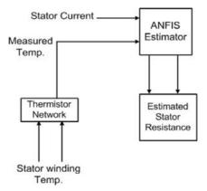
Figure 16. Block diagram of stator resistance estimation using ANFIS estimator
