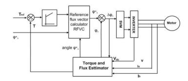
Figure 4. System Diagram of the Modified DTC IM Drive
