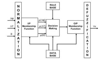
Figure 15. DTFC functional block diagram
