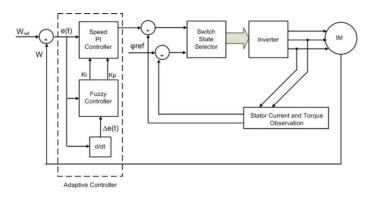
Figure 11. Fuzzy PI-Controller based DTC
