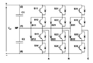
Figure 6. Three level neutral point clamped voltage source inverter
