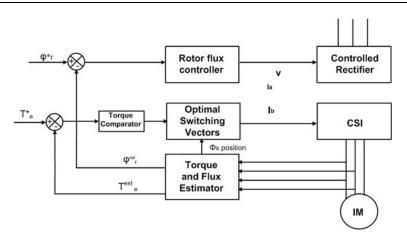
Figure 7. Basic scheme of DTC CSI-fed IM drive
