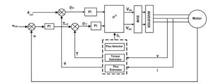
Figure 2. Modified DTC Scheme- 1 Block Diagram
