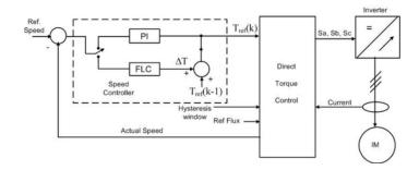
Figure 10. DTC system with PI and FLC controller for speed loop
