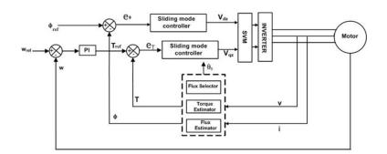
Figure 3. Modified DTC Scheme-2 Block Diagram
