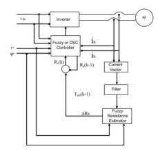
Figure 12. Direct torque control with fuzzy resistance estimator
