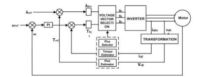
Figure 1. Block Diagram of DTC
