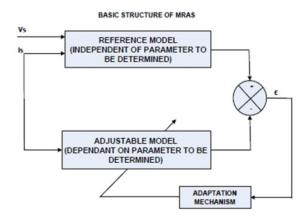
Figure 13. MARS based stator resistance estimation scheme
