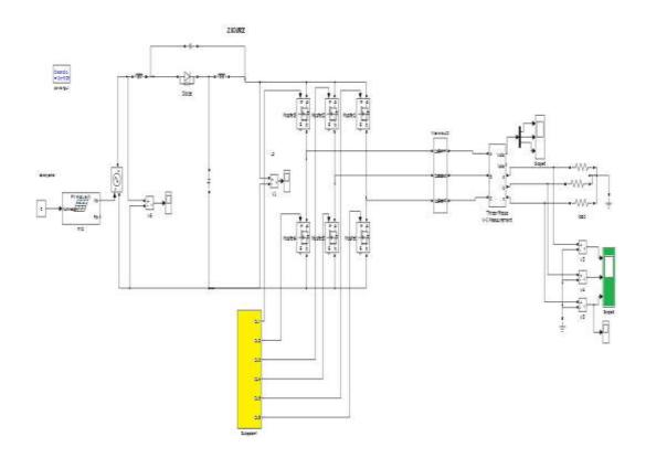
Figure 11. Quasi Z-Source Inverter using SVM
