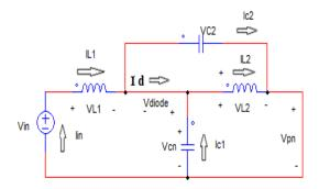
Figure 3. Non-Shoot through Equivalent Circuit
