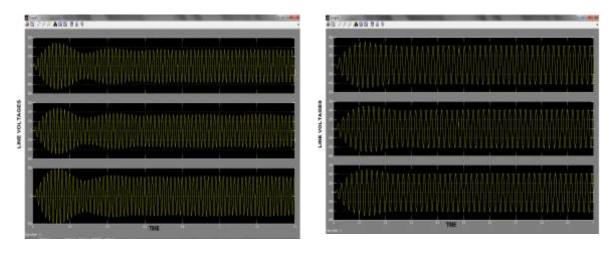
Figure 7. Output waveform of Quasi Z source Inverter for SPWM Technique
