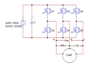
Figure 4. Three Phase Inverter
