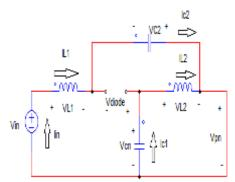
Figure 2. Shoot through Equivalent Circuit
