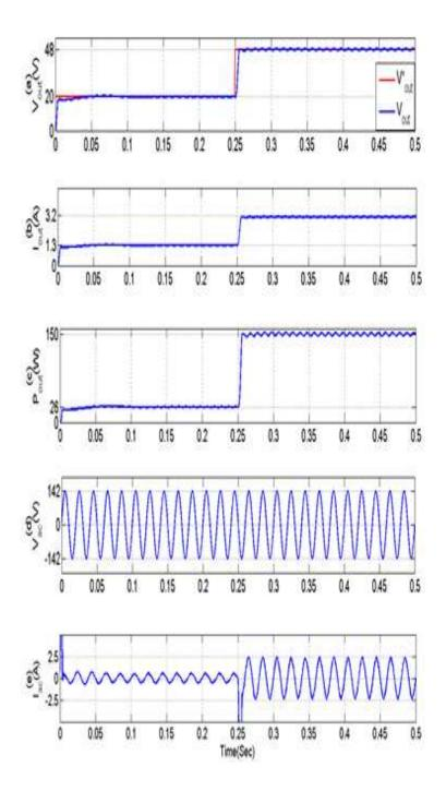
Figure 8. The dynamic performance of the proposed converter during different values of output voltage
