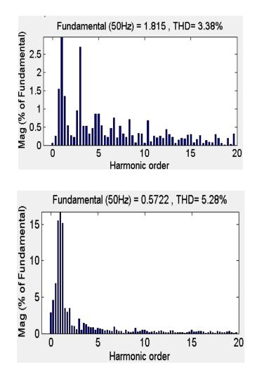
Figure 9. Harmonic spectra of supply current at rated input supply on LED Lamp and output voltage as (a) 48 V and (b) 20 V.
