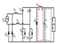
Figure 3(c). Mode 2 operation during a complete switching period for the positive half-cycles of the supply voltage
