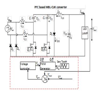
Figure 2. The proposed PFC (Modified Bridge Less-CUK) MBL-CUK converter
