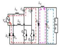
Figure 3(b). Mode 1 operation during positive half-cycles of the supply voltage
