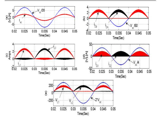
Figure 7(a -e). A sinusoidal supply current in phase with supply voltage
