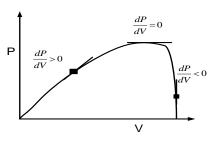
Figure 2. P-V characteristics of solar cell
