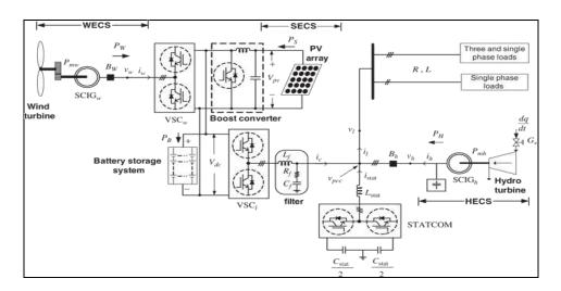
Figure 4. Proposed model for hybrid energy system with solar, wind and small hydro resources
