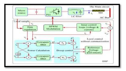
Figure 5. Control structure of conventional P/f and Q/V droop control
