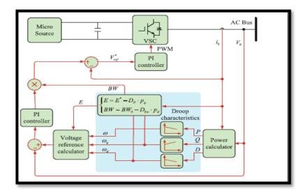
Figure 6. Proposed Block diagram of the frequency signal injection method
