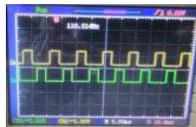
Figure 4.5. Switching Pulse for M1, M3 of Inverter
