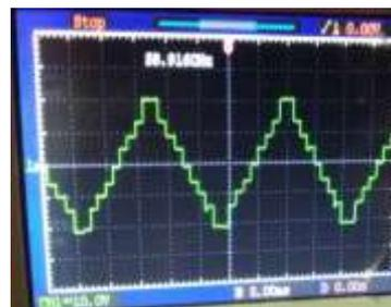
Figure 4.9. Output Voltage of MLI
