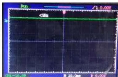
Figure 4.4. Output Voltage of Boost to SEPIC
