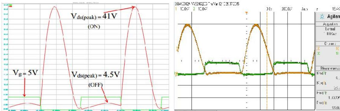
(c) Circuit Experiment ( $R_L < R_{opt}$ ): Switch Voltage
