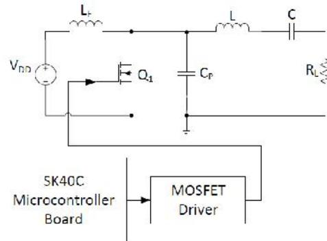
Figure 5. Class-E Power Amplifier with MOSFET Driver Circuit
