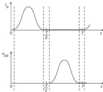
Figure 1. (a) Current Through Switch (b) Voltage Across Switch [13]
