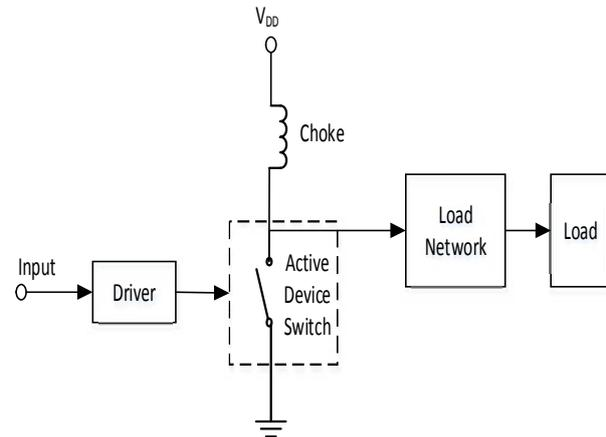
Figure 2. Single-ended Switch-mode Power Amplifier Block Diagram
