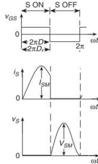
Figure 4. Theoretical Waveforms in Class E zero-voltage-switching amplifier [13]
