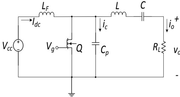
Figure 3. Typical Class-E Power Amplifier Circuit
