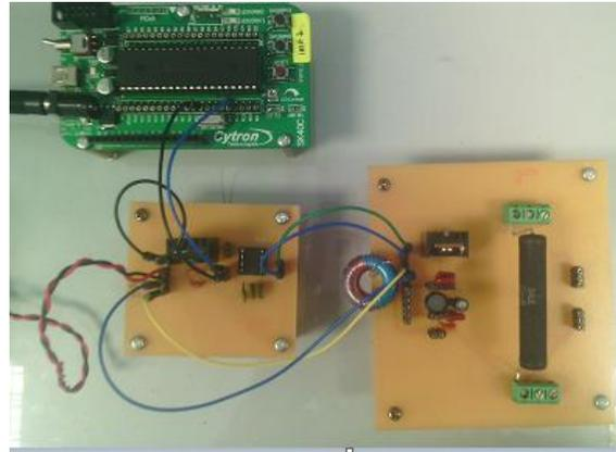
Figure 6. Class-E Power Amplifier Experimental Setup
