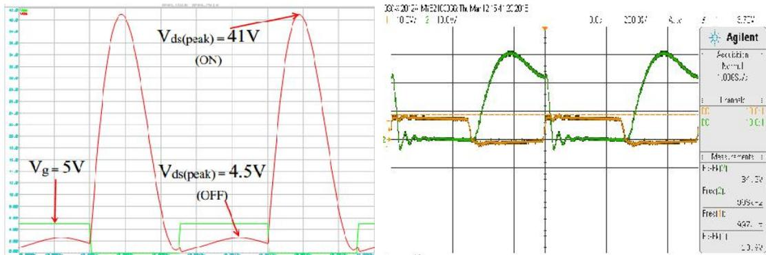
(a) Circuit Experiment ( $R_L > R_{opt}$ ): Switch Voltage
