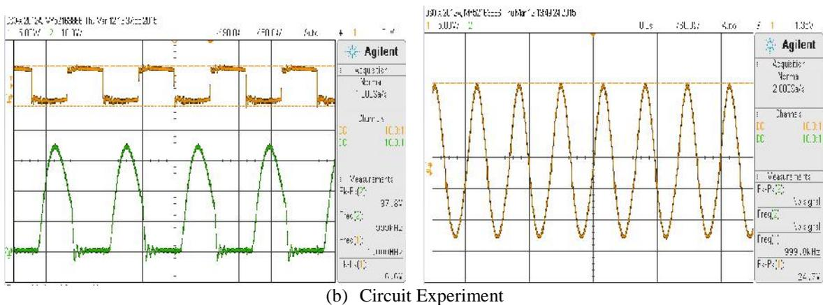
Figure 7. Input, Switching Voltage and Output Voltage Waveforms for the First Design at 1MHz Frequency
