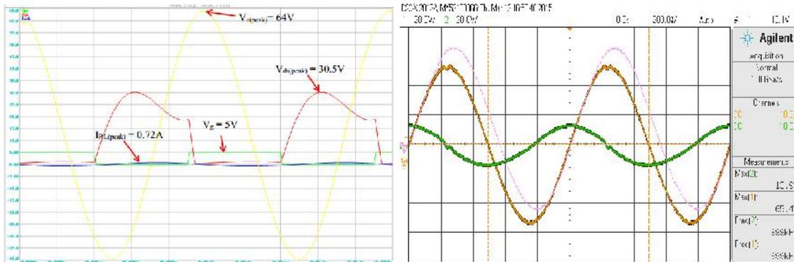
(b) Circuit Experiment ( $R_L > R_{opt}$ ): Capacitor Voltage
