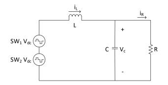
Figure 4. Simplified equivalent average circuit of the 5-level CHMI
