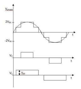
Figure 2. 5-level CHMI with LC filter
