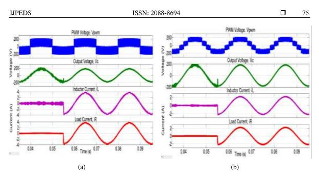
Figure 5. No load to full load condition, top to bottom, PWM voltage  $V_{PWM}$ , output capacitor voltage  $V_C$ , inductor current  $i_L$ , and load current  $i_R$  (a) H-bridge Inverter and (b) 5-level CHMI
