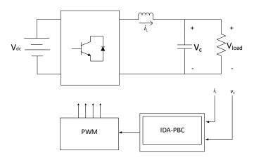
Figure 1. Inverter controlled by the IDA-PBC
