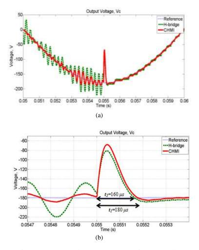
Figure 6. Comparison of output voltage waveform during no load to full load condition showing ripples and transient time, t<sub>1</sub> and t<sub>2</sub> (a) Ripples (b) Transient time
