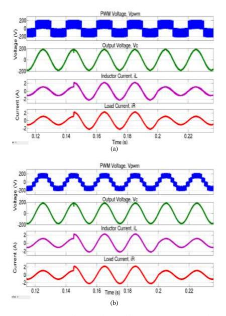
Figure 7. System response under transient operating conditions, top to bottom, PWM voltage  $V_{PWM}$ , output capacitor voltage  $v_C$ , inductor current  $i_L$ , and load current  $i_R$  (a) H-bridge Inverter and (b) 5-level CHMI
