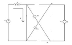
Figure 2. Equivalent circuit of diode assisted buck-boost converter during S1 is ON
