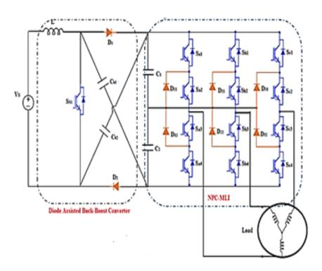
Figure 1. Circuit diagram of diode assisted buck-boost converter with NPC-MLI
