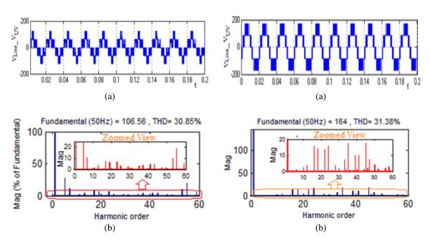
Figure 6. output performance characteristics for M<sub>a</sub>=0.7 (a) Line voltage (b) THD spectra
