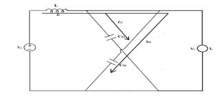
Figure 3. Equivalent circuit of diode assisted buck-boost converter during S<sub>1</sub> is OFF
