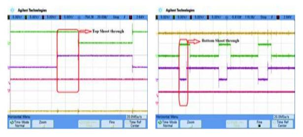
Figure 8. Gate pulses of one leg in top shoot through
