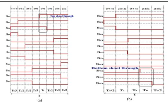
Figure 5. Switching operation of NPC-MLI (a) Top shoot through (b) Bottom shoot through
