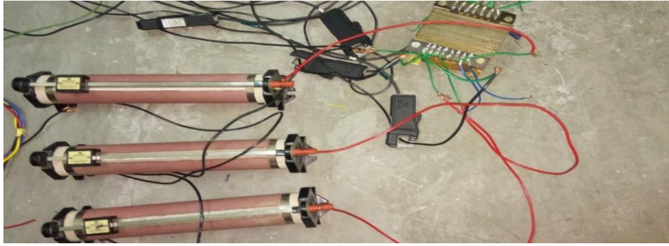
Figure 15. Resistive and Inductive Load Used for Testing The Results
