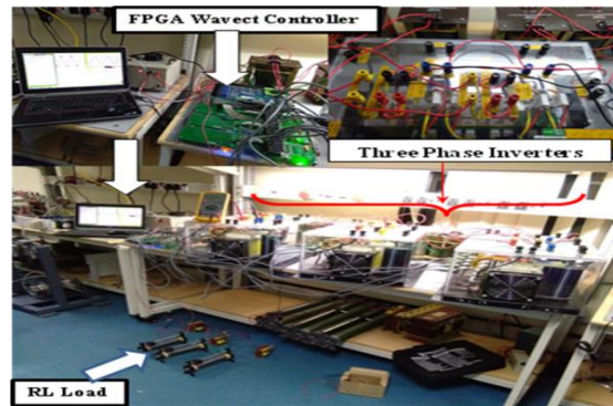
Figure 7. Hardware Setup of three-phase cascaded multilevel inverter with Semikron kit and WAVECT software
