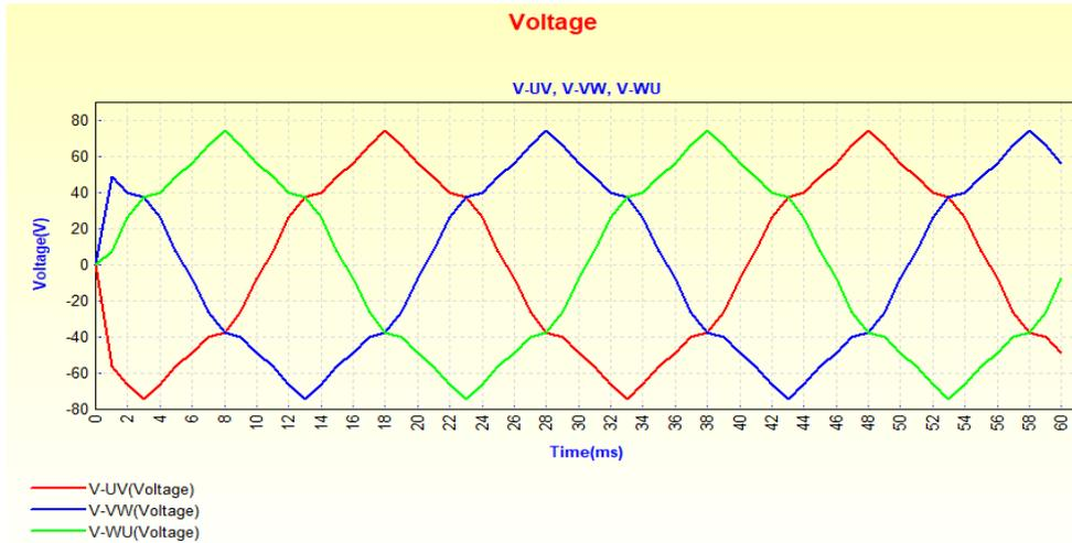
Figure 4. Line to line voltage by FEM software method
