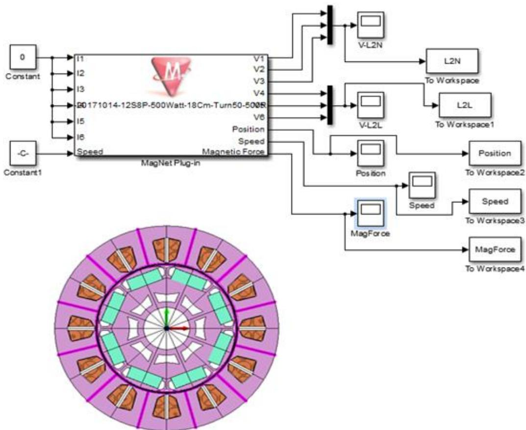
Figure 2. Electrical permanent magnet generator design with Co-Simulation Magnet/Simulink software
