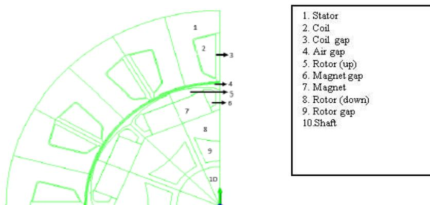
Figure 1. Geometry designed of electric generator
