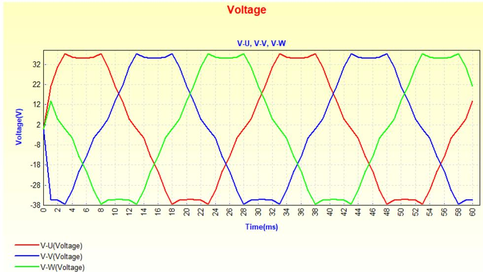
Figure 6. Line to neutral by FEM software method
