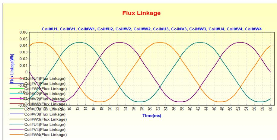
Figure 3. Flux linkage each coil by FEM software method
