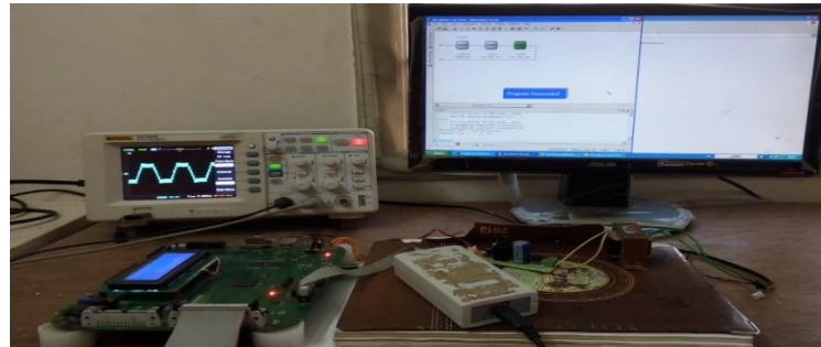
Figure 12. VHDL Code Successfully Embedded in FPGA for 1- \phi Seven-Level CBRV Inverter
