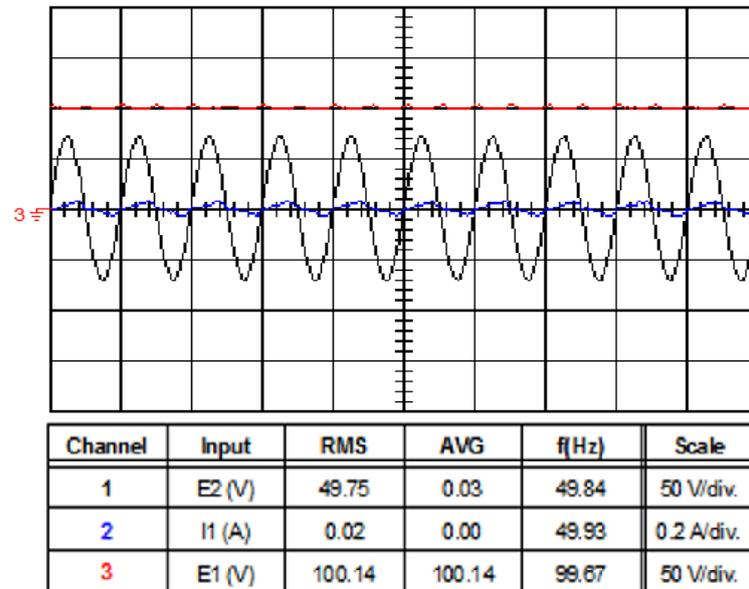
Figure 6. Input voltage input current and output dc voltage
