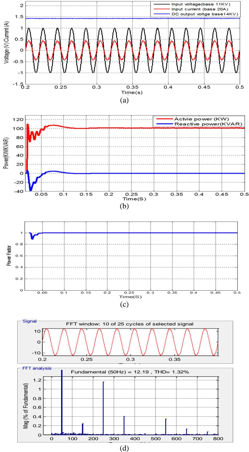
Figure 3. (a) Input voltage, input current and output dc voltage, (b) Active and reactive power, (c) Input power factor and (d) THD on the grid side
