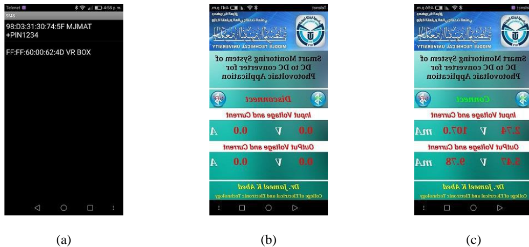
Figure 9. Windows of DC/DC Converter Application: (a) HC-5 Bluetooth Searching Window; (b) Main Application Window Before Bluetooth Connected; (c) Main Application Window with Results after Bluetooth Connected
