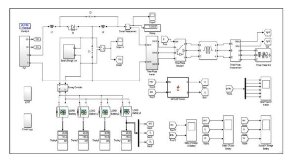
Figure 3. Overall MATLAB circuit diagram for bidirectional vehicle charging station using qZSI PV inverter
