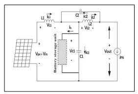
Figure 1. Equivalent circuit of shoot through state
