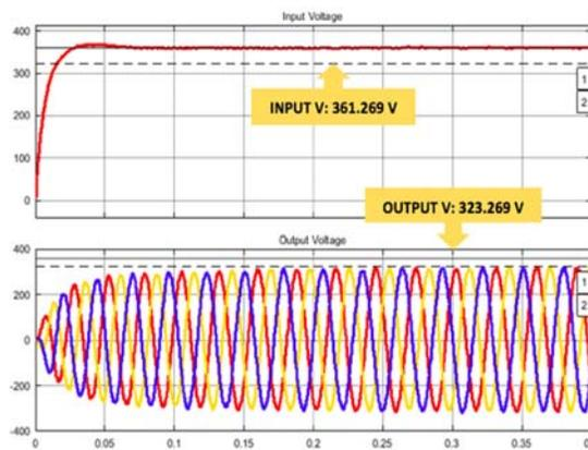
Figure 6. Input and output voltage with 100kW load
