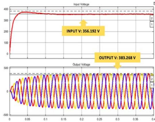
Figure 5. Input and output voltage with 50kW load
