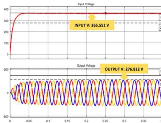
Figure 7. Input and output voltage with 150kW load
