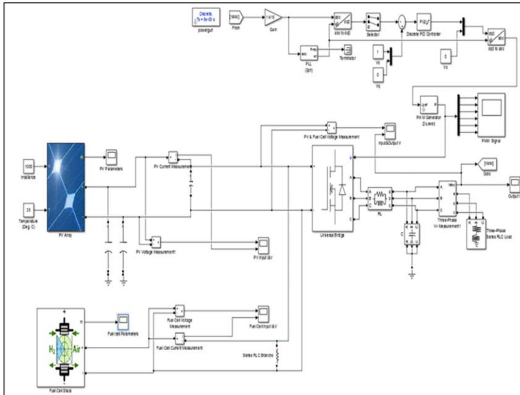
Figure 3. MATLAB/Simulink circuit design for control of hybrid AC microgrid
