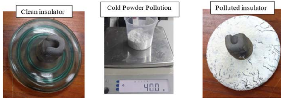
Figure 4. Glass insulator and pollution
