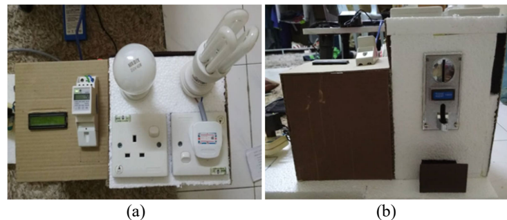
Figure 4. Prototype coin kWh meter, (a) top view, (b) front view
