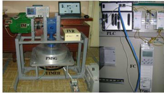
Figure 5. Stand for the testing of CHP WECS
