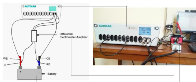
Figure 1. Schematic of the electrochemical test setup using metrohm autolab potentiostat in two electrodes set up, RE=reference electrode, WE=working electrode, and S=signal (left). The real experimental setup during the battery charging and discharging process (right)
