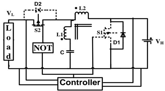
Figure 4. Conductions states of S1, D1, S2, and D2 in boost mode of circuit shown in Figure 2
