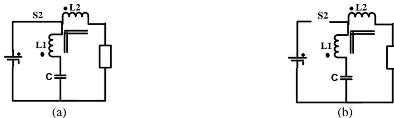
Figure 6. Switching state of S2 of (a) ON state of S2 and (b) OFF state of S2
