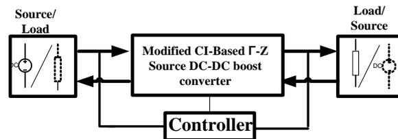
Figure 1. Block diagram of proposed modified CI-based Bi-directional DC-DC buck-boost converter
