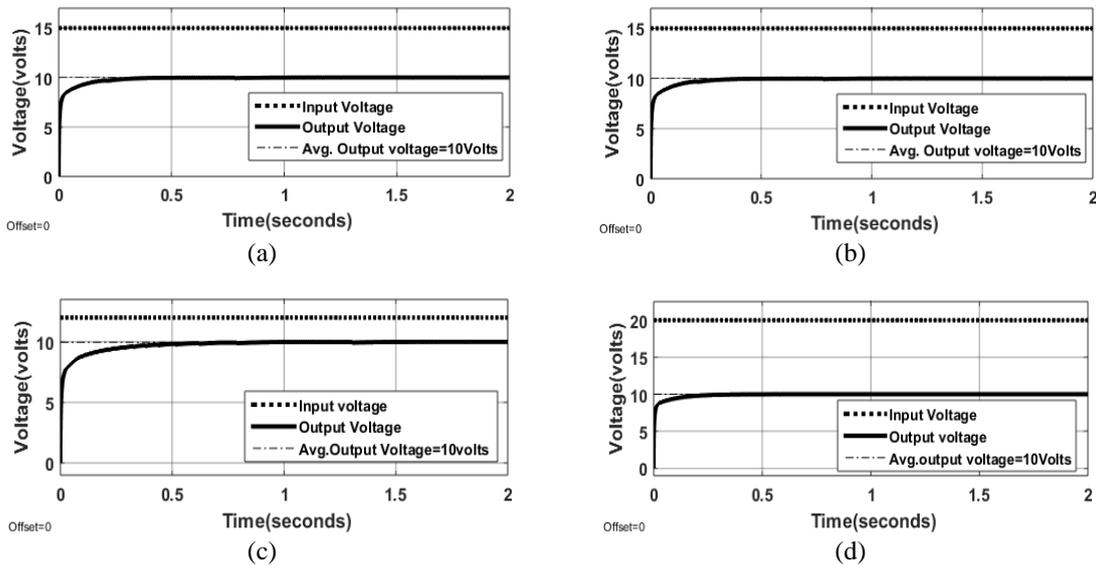
Figure 10. Output voltage (vs) input voltage graphs to verify gain sensitivity of proposed converter in buck operating mode, (a) for  $V_{dc}$  @ 15 V &  $R_L$  @ 200  $\Omega$ , (b) for  $V_{dc}$  @ 15 V &  $R_L$  @ 700  $\Omega$ , (c) for  $V_{dc}$  @ 12 V &  $R_L$  @ 200  $\Omega$ , and (d) for  $V_{dc}$  @ 20 V &  $R_L$  @ 700  $\Omega$
