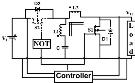
Figure 3. Conductions states of S1, D1, S2, and D2 in boost mode of circuit shown in Figure 2
