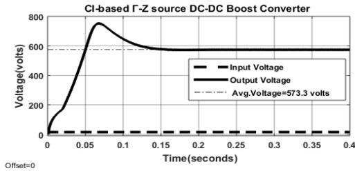
Figure 7. Input and output voltages of proposed converter in boosting mode
