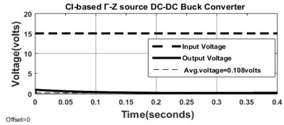
Figure 8. Input and output voltages of proposed converter in buck mode
