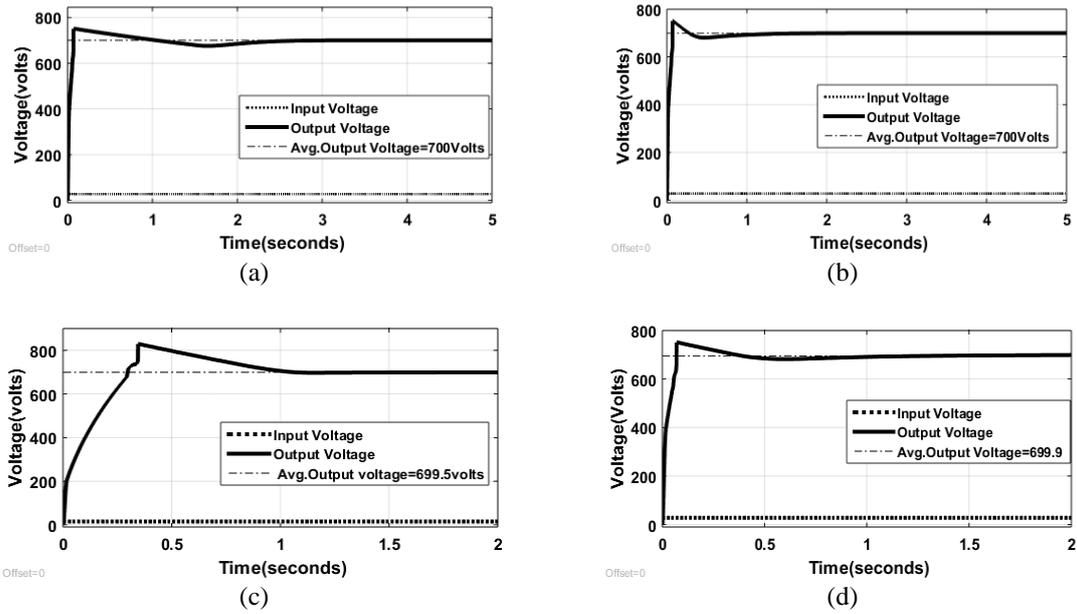
Figure 9. Output voltage (vs) input voltage graphs to verify gain sensitivity of proposed converter in boost operating mode, (a) for  $V_{dc}$  @ 15 V &  $R_L$  @ 200  $\Omega$ , (b) for  $V_{dc}$  @ 15 V &  $R_L$  @ 700  $\Omega$ , (c) for  $V_{dc}$  @ 12 V &  $R_L$  @ 200  $\Omega$ , and (d) for  $V_{dc}$  @ 12 V &  $R_L$  @ 700  $\Omega$
