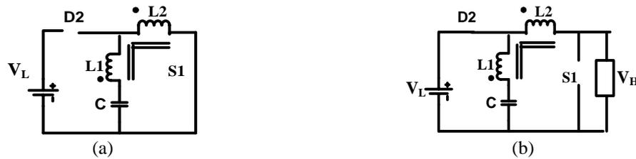
Figure 5. Switching states of S1 and D2 in (a) S1-ON and D2-OFF and (b) S1-OFF and D2-ON
