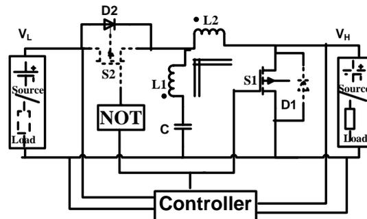
Figure 2. Circuit diagram of proposed CI-based Bi-directional DC-DC buck-boost converter
