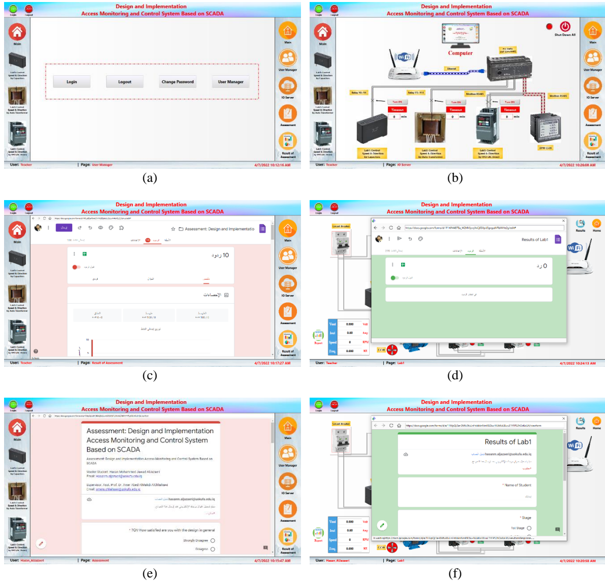
Figure 3. Windows of the system (a) user manager, (b) IO server, (c) assessment, (d) result of assessment, (e) report, and (f) results
