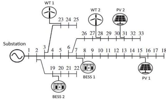
Figure 5. The optimal location results in the IEEE 33 bus network
