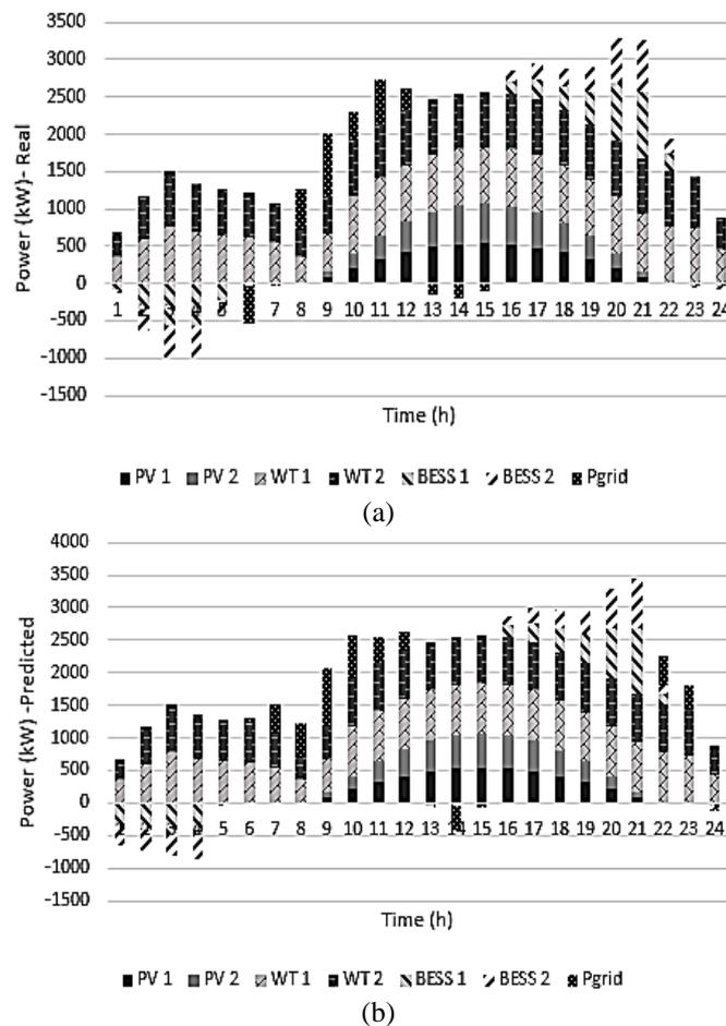
Figure 9. Optimal energy distribution decisions for (a) case 1 and (b) case 2
