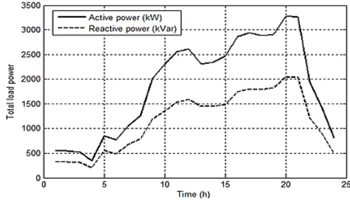
Figure 3. Typical load profile
