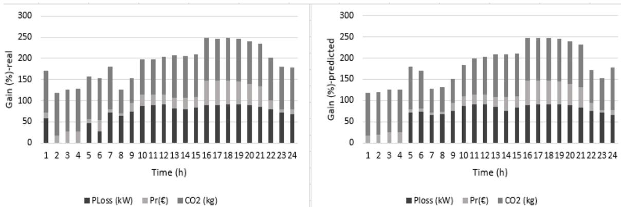
Figure 11. Gains in terms of power losses, profits and CO<sub>2</sub> emissions
