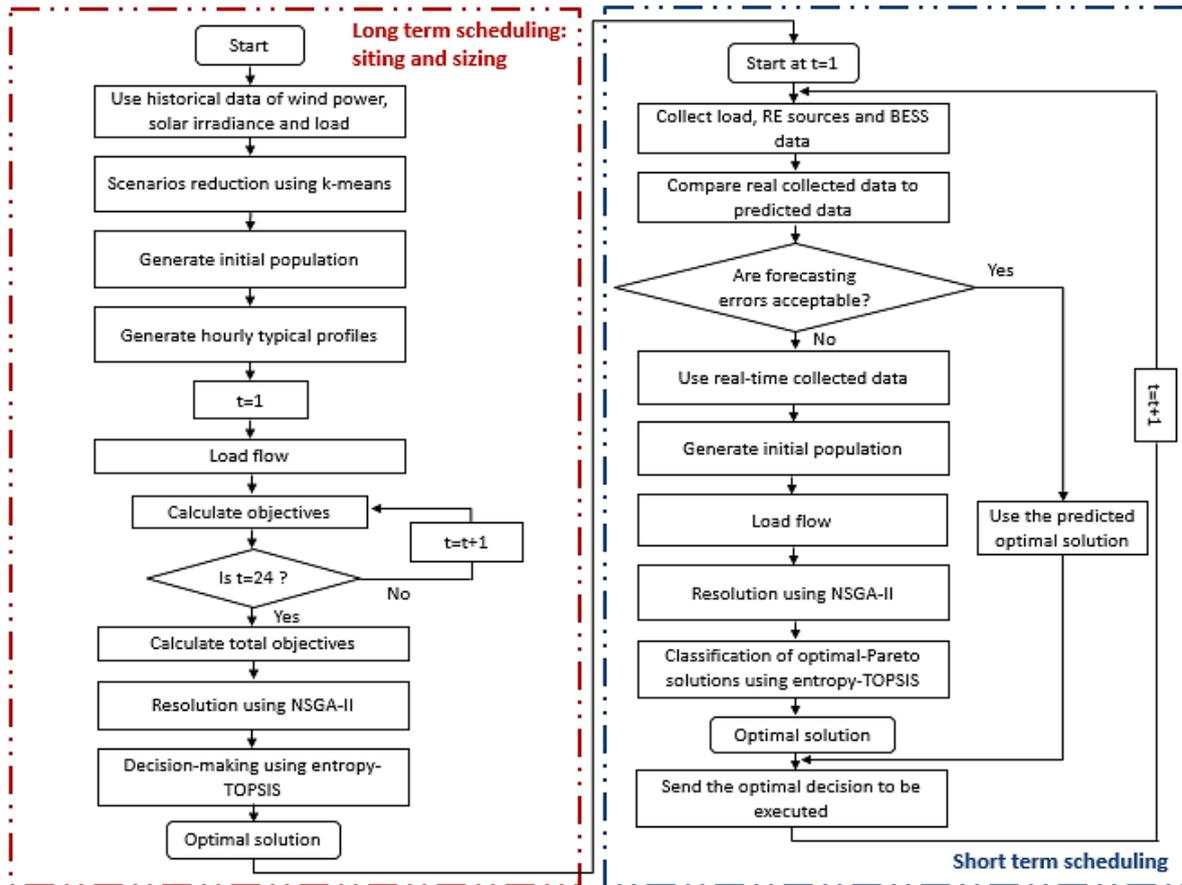
Figure 2. The two-level scheduling solution flowchart
