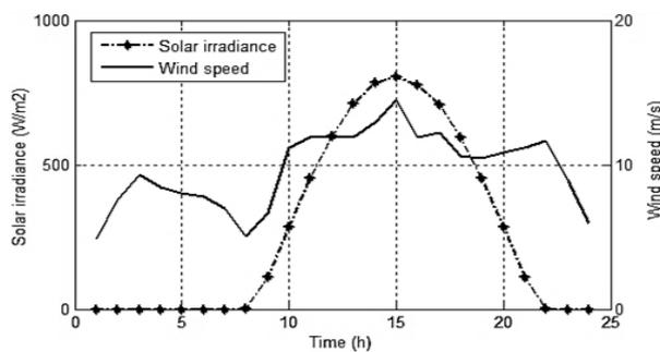
Figure 6. Wind speed and solar irradiance data for a sunny day
