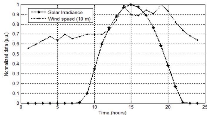
Figure 4. Normalized typical data of wind speed and solar irradiance
