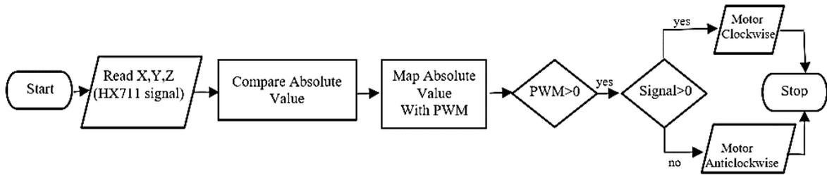
Figure 7. Algorithm used to reduce crosstalk
