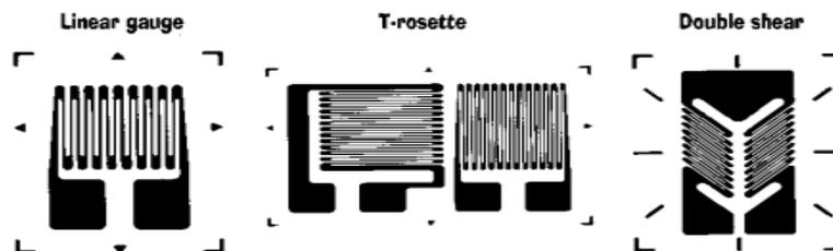
Figure 1. Type of strain gauges
