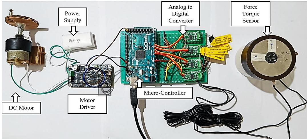
Figure 4. Experimental setup
