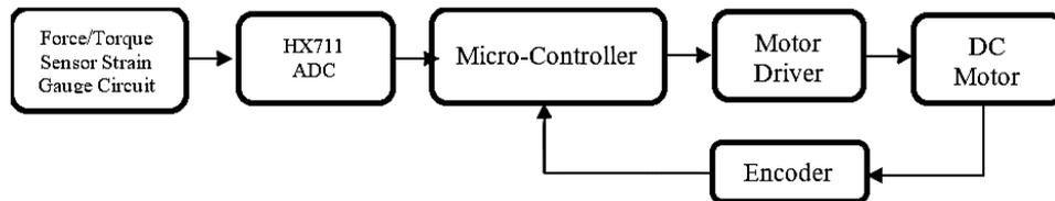
Figure 3. Block diagram of data acquisition
