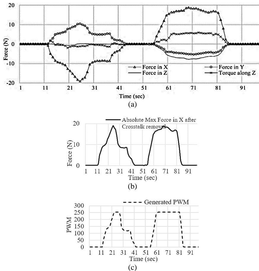
Figure 8. Crosstalk removal (a) data collected, (b) mapped absolute value, and (c) generated PWM
