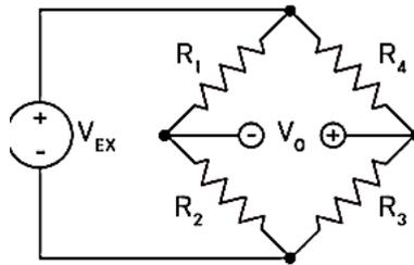
Figure 2. Wheatstone bridge circuit configuration in rhombus style
