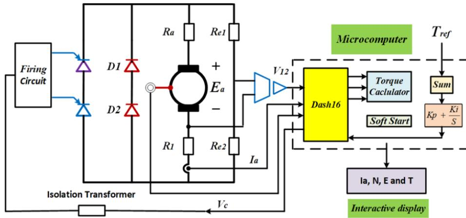
Figure 13. Block diagram of PC-based torque controller for DC motor
