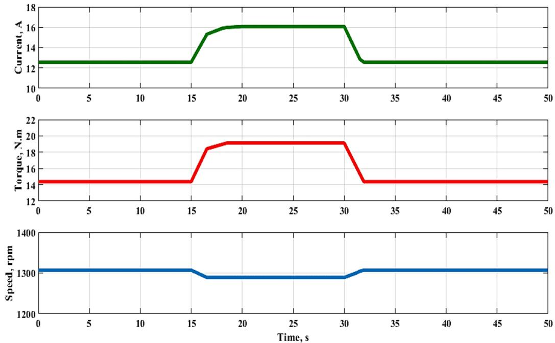
Figure 10. System simulation waveform with P-controller ( $K_P = 1.5$ )
