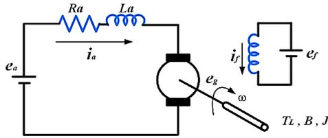
Figure 1. DC separately excited motor
