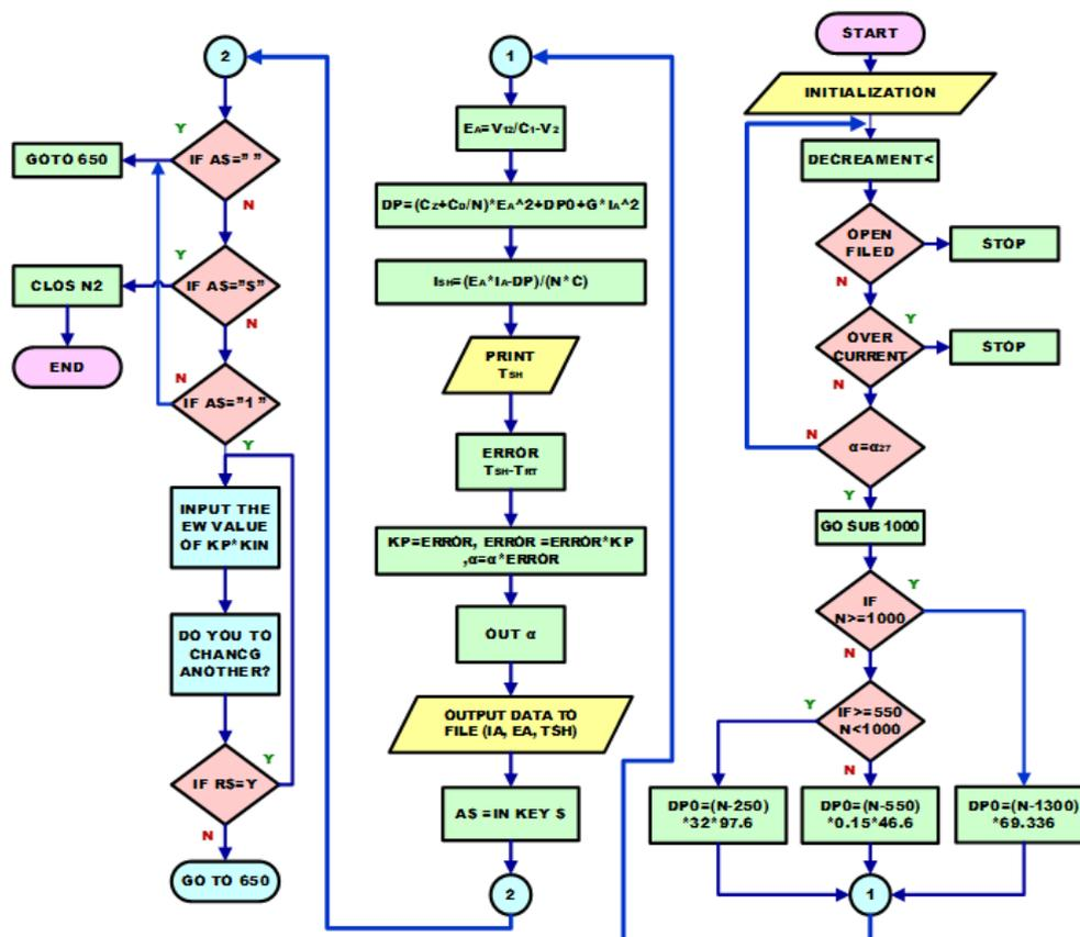
Figure 17. Flow chart for the microcomputer-based torque control
