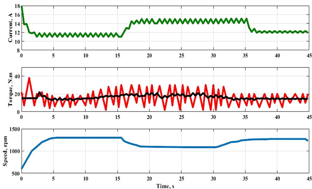
Figure 19. System waveform with P controller ( $K_P = 1.5$ )
