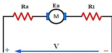
Figure 3. Equivalent circuit of DC machine
