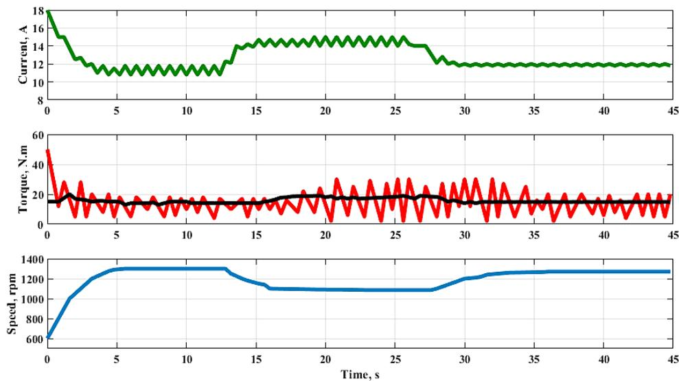
Figure 18. System waveform with P controller ( $K_P = 0.9$ )
