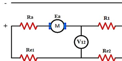
Figure 4. EMF bridge measurement
