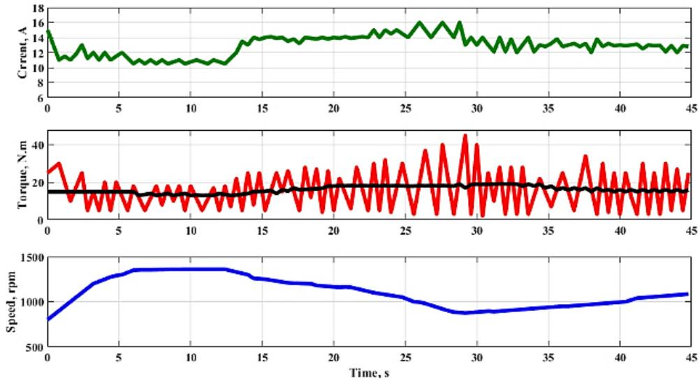
Figure 20. System waveform with PI controller ( $K_P = 0.9$ ,  $K_I = 0.01$ )
