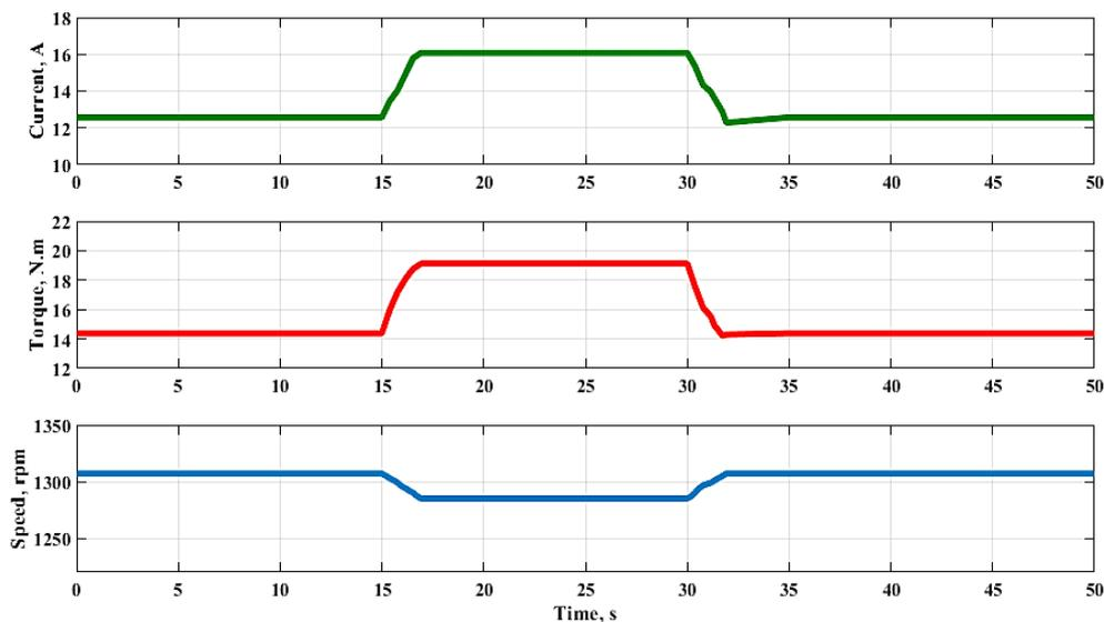
Figure 8. System simulation waveform with P-controller (KP = 1)
