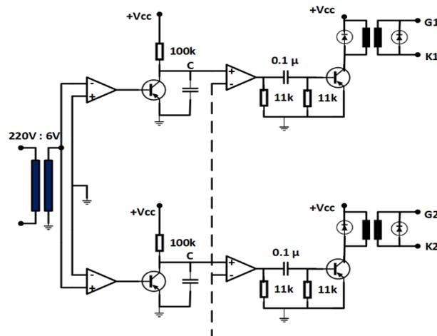
Figure 16. The firing circuits
