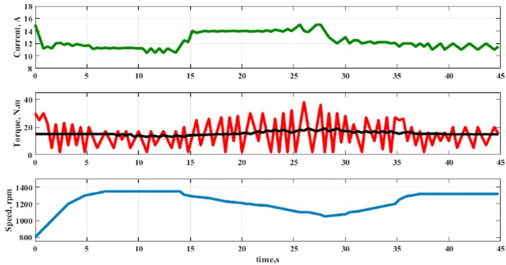
Figure 21. System waveform with PI controller ( $K_P = 0.9$ ,  $K_I = 0.0161$ )
