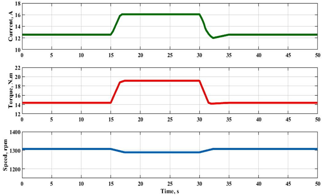
Figure 9. System simulation waveform with P-controller ( $K_P = 1.2$ )
