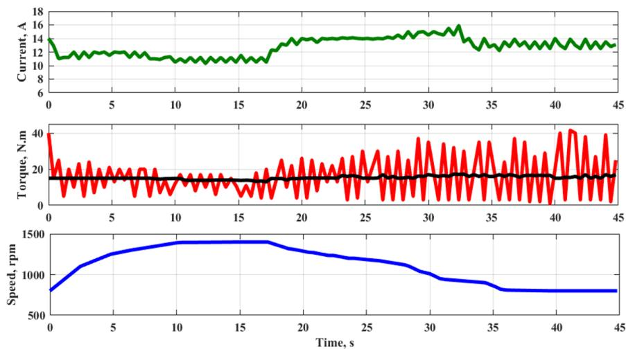
Figure 22. System waveform with PI controller ( $K_P = 0.6$ ,  $K_I = 0.02$ )
