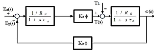
Figure 2. The block diagram transfer function of DC motor torque control
