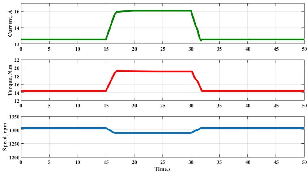
Figure 7. System simulation waveform with P-controller (KP = 0.9)
