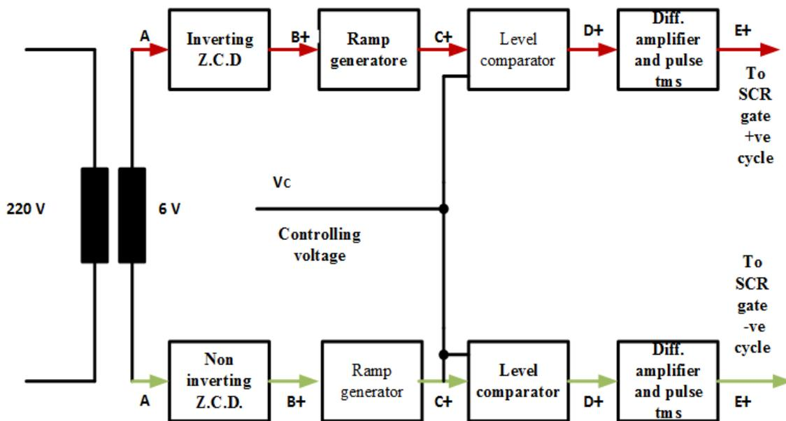
Figure 15. Block diagram of the firing circuit
