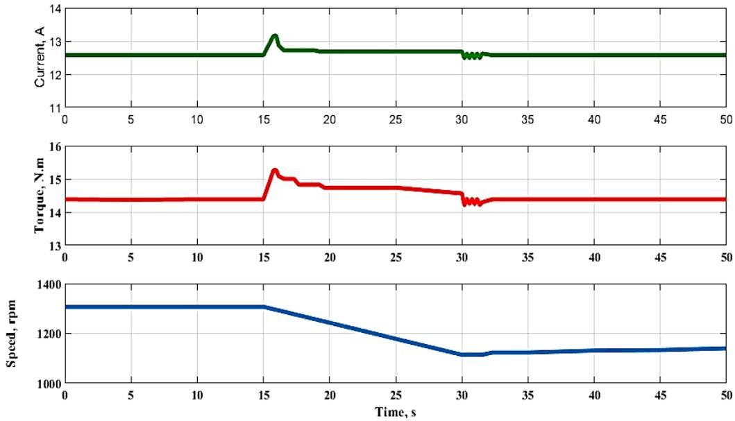
Figure 11. System simulation waveform with PI-controller ( $K_P = 0.9$ ,  $K_I = 0.022$ )
