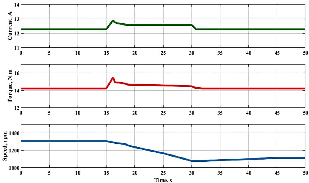
Figure 12. System simulation waveform with PI-controller ( $K_P = 0.9$ ,  $K_I = 0.025$ )
