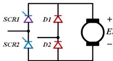
Figure 14. Single phase half-controlled bridge
