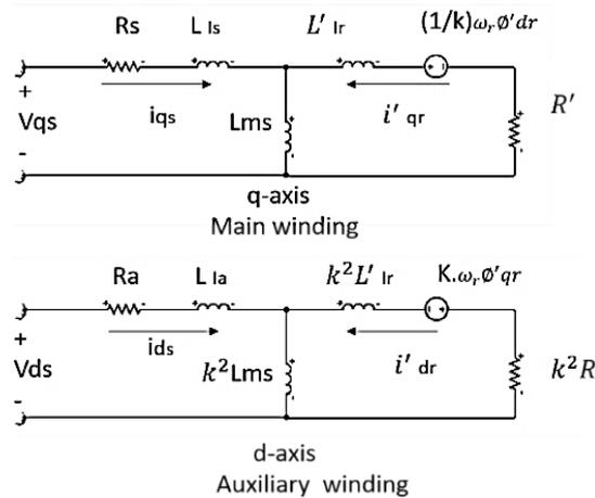
Figure 5. Equivalent circuit of unsymmetrical 1-Φ induction motor (stationary reference frame)
