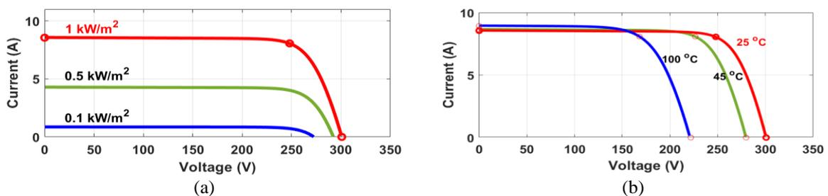
Figure 7. V-I characteristics of Trina Solar TSM-250PA05.08 array type: (a) array @ 1000 W/m<sup>2</sup> and specified irradiation; and (b) array @ 25° and specified irradiation
