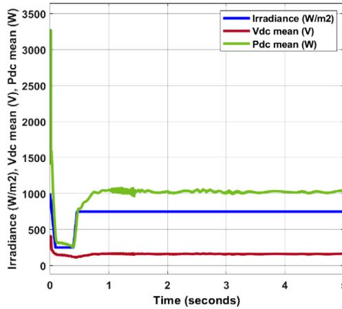
Figure 9. Absorbed irradiance by the PV array in (w/m<sup>2</sup>), mean DC voltage in (v) and mean power in (w) generated by PV array
