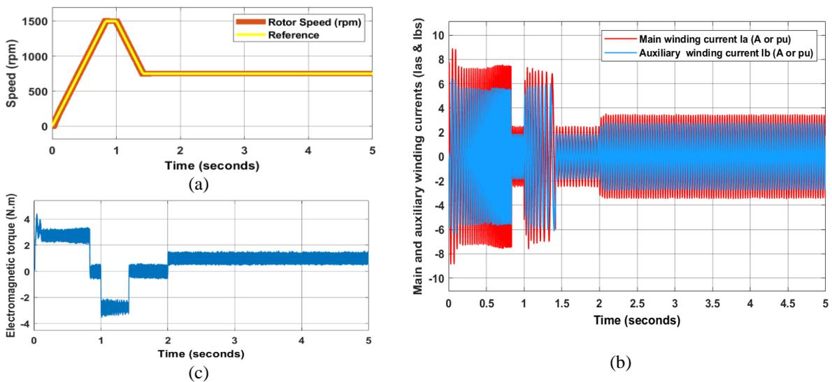
Figure 10. 1-Φ induction motor simulation results (a) rotor speed, (b) main and auxiliary winding currents, and (c) electromagnetic torque  $T_e$
