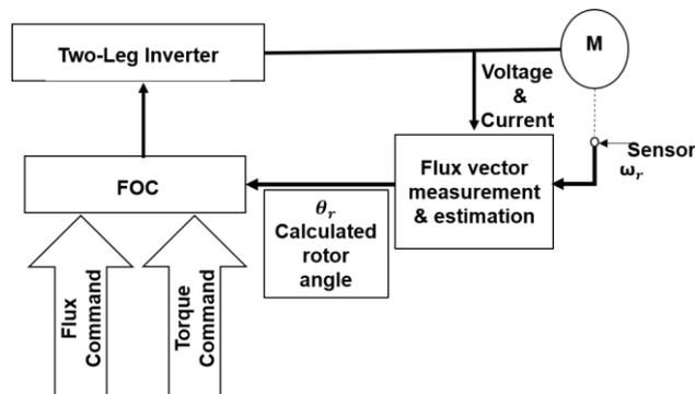
Figure 6. Diagram of FOC for 1-Φ induction motor
