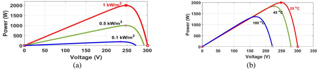
Figure 8. V-P characteristics of TSM-250PA05.08 array type: (a) array @1000 W/m<sup>2</sup> and specified irradiation; and (b) array @25° and specified irradiation
