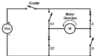
Figure 2. Full h-bridge schematic
